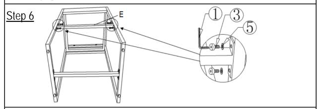
Attach Footrest (E) between the Legs using Bolts(③) and Washers(⑤) with Allen Key(①). **Do not fully tighten the Bolts.**
