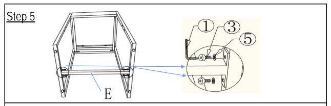
Attach Footrest (E) between the Legs using Bolts(③) and Washers(⑤) with Allen Key(①). **Do not fully tighten the Bolts.**
