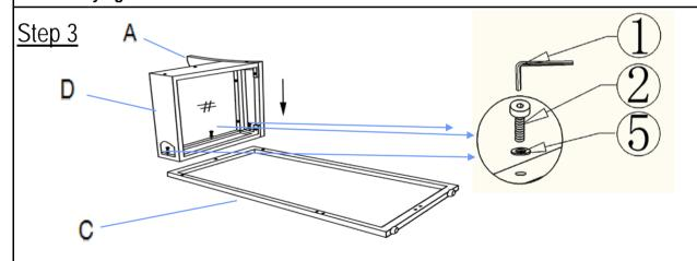
Attach Left Leg(C) to Backrest(A) and Seat Panel(D) using Bolts(2) and Washers(5) with Allen Key(1).
