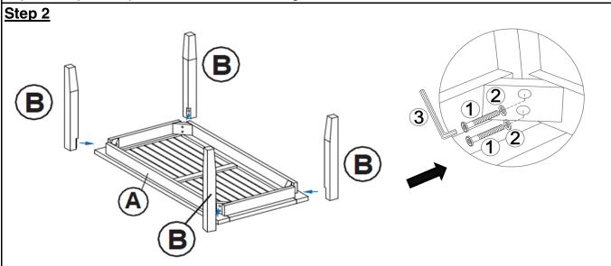
Place the Table top (A) with its underside skywards onto a clean, soft surface to avoid any scratch or damage to the product.
