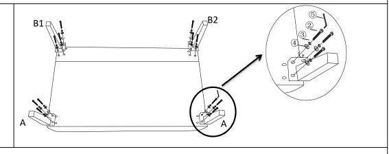
Install the legs(A&B1&B2) to Seat by using the Medium Bolt (②) + Spring Washer (③) + Washer(④) as shown. Use the Allen Key(⑤) to fasten all bolts. Caution:Do not fully tighten.
