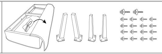
REMOVE the non-woven fabric from under the seat, take out the legs and hardware accessories.
