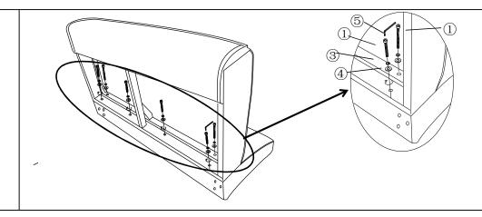
Put the Backrest onto a flat table or panel, insert the positioning dowels on the Seat panel to the mounting positionon the Backrest panel.
