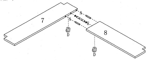
Assemble the long shelf (7) and short shelf (8) by wooden dowel (A), double head bolt (E) and cam lock (D).
