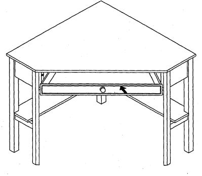
Slide the drawer at an angle to fix to wooden drawer glide (9).
