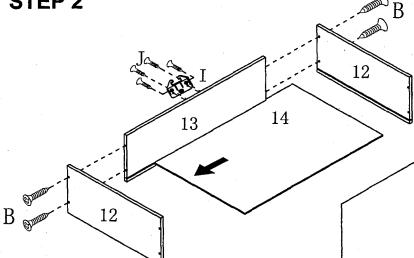
Assemble drawer plastic glide (I) to drawer backpanel (13) by using screw (J);
