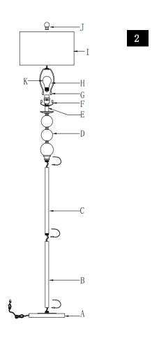
Step2 Insert the Harp (H) into the Saddle (F). tighten the Finial (J)into the Harp (H) Insert the bulb(K) into the socket(G).
