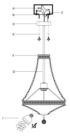
PLEASUE USE ON/OFF TYPE"A" BULB MAX 60-WATT OR CFL BULB MAX 23-WATT THERE IS CFL 13-WATT BULB IN THE BOX.
