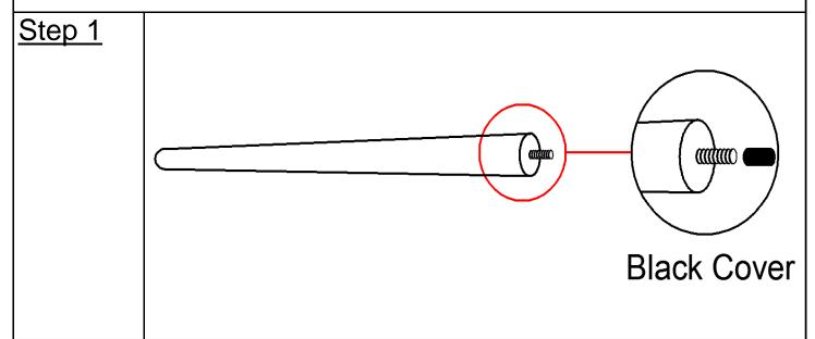
Open the carton and place all parts onto a clean, non-marring surface. Remove the Black Cover on the threaded stem of the Legs(B).
