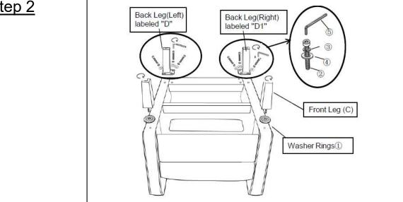
Install the Front Leg(C) and Back Leg(Left&Right) into the bottom of the Chair Base Body(B) by placing a Washer Ring (1)Bolt(2)Spring WasherRing(③)Flat Washer Ring(④) with Allen Key(⑤)onto the threaded stem. And then insert the threaded Stem into the threaded Mounting Position ateach Corner of the Bottom of the Chair.
