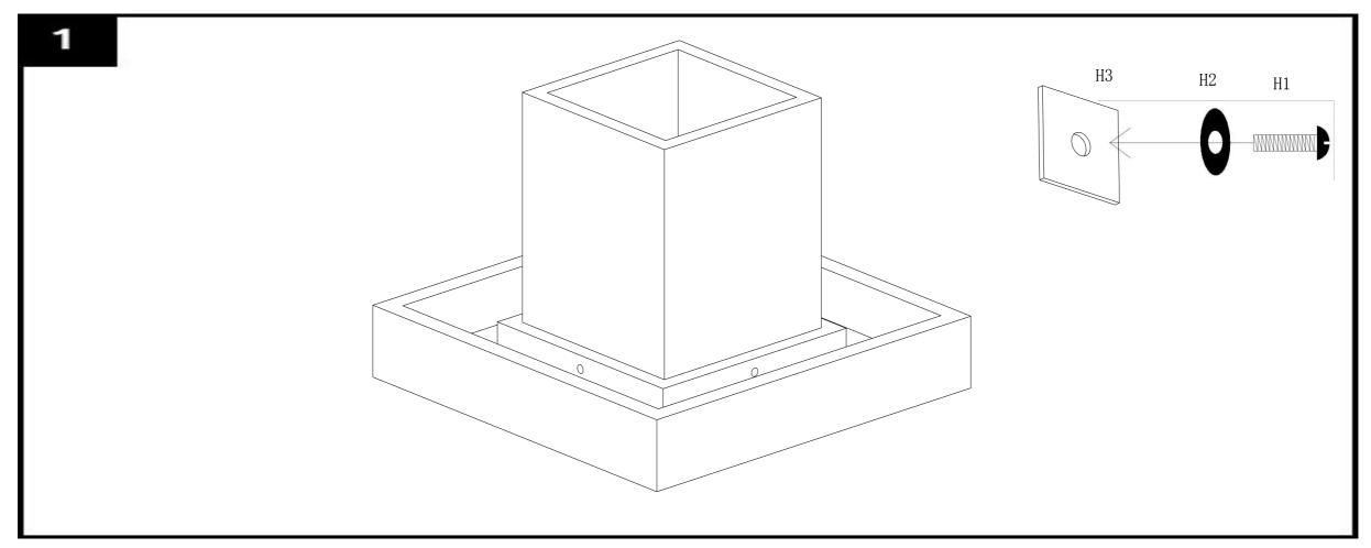
Step 1: Use allen key (H4) to tight the bolt M8(H1) to press on plastic plug that is fixed into concret base. Tighten the bolt untill it touches the plastic plug without piercing
