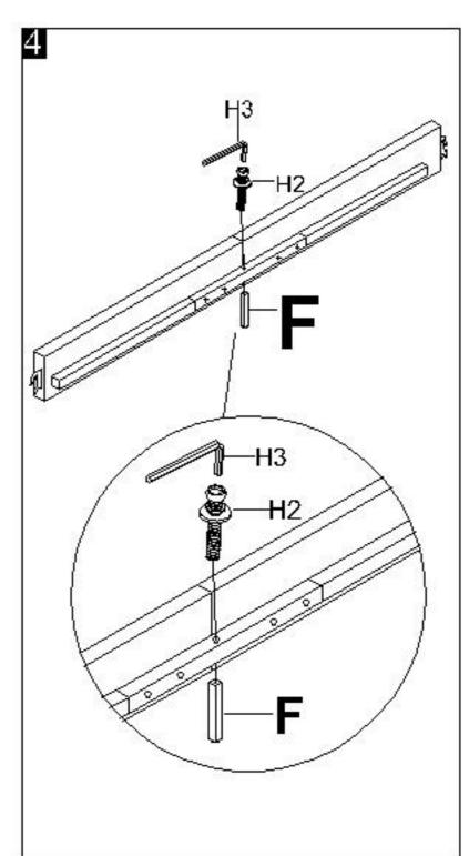
Attach support legs "F" to wood bar "K" .Using wrench (H3) to lock with bolts "H2".
