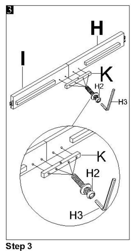
Attach wood bar "K" to the 2 rails "H" & "I". Using wrench (H3) to lock with bolts "H2".
