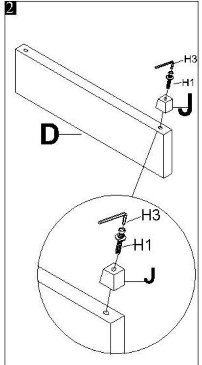
Attach wood legs "J" with footboard "D". Using wrench (H3) to lock with bolts "H1".
