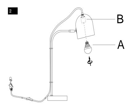
Step 2 Insert the Bulb(A) into the socket.
