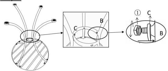
Attach the Support Ring(C) to Table Legs(B) using Nuts(1) with Spanner(2). **Loosely tighten Nuts.**
