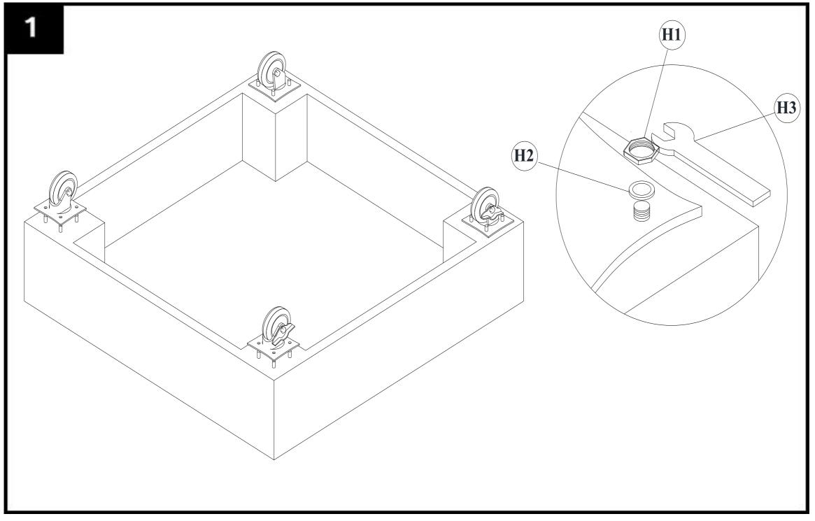
Step 1: The hardware need to connect wheels (B), (C) and concrete top are 16 nut (H1) and washer (H2)
