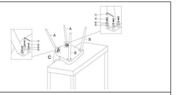
Attach Hind Leg(A) to Chair Seat(C) using Bolts(2), Washers(3), and Spring Washers(4), with Allen Key(1) as pictured above.
