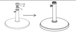
For the Umbrela Pole with diameter as 48mm, use the Dia. 48mm Adapter (I) only, insert the Dia. 48mm Adapter (I) into the Support Pole (E).
