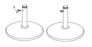
Screw the Adjustable Screw (F) into the Support Pole(E).
