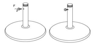
Screw the Adjustable Screw (F) into the Support Pole (E).
