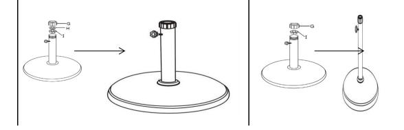
For the Umbrela Pole with diameter as 35mm, use Dia. 35mm Adapter (H) & Dia. 38mm Adapter (I) added together, insert the Dia. 38mm Adapter (I) into the Support Pole (E) first, and then put the Dia. 35mm Adapter (H) onto the Dia. 38mm Adapter(I). Turn the Cap(G) onto the Support Pole(E) to hold the Adapters in place.
