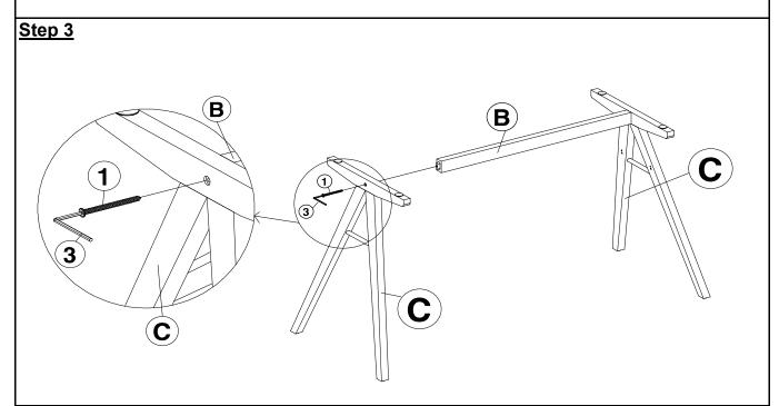
Repeat same process as Step 2 to attach the Horizontal support bar (B) with another Leg (C) as shown in picture.
