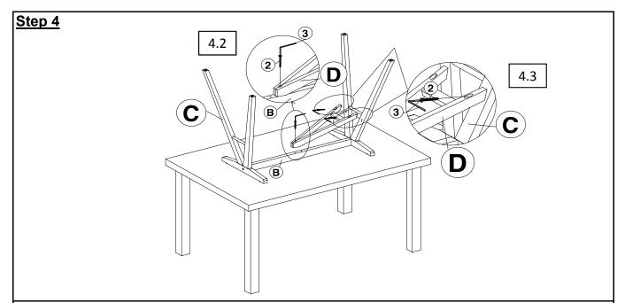
Step 4.1: Place the assembled frame face skywards onto a clean, soft surface to avoid any scratches or damages to the product. Then attach the Support bar (D) into assembled frame as shown in picture.
