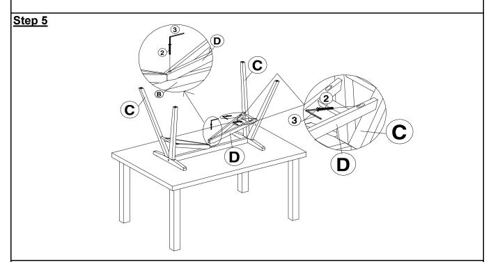
Repeat same process as Step 4 to attach the Support bar (D) with assembled frame as shown in picture.
