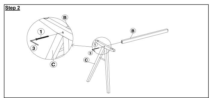
Attach the Horizontal support bar (B) with the Leg (C) as shown in picture.
