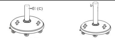
Screw Adjustable Screw(C) into Support Pole(B).
