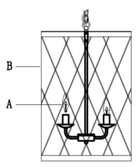
PLEASE USE ON/OFF TYPE"B" BULB MAX 40-WATT OR CFL BULB MAX 9-WATT THERE ARE 5PCS 25-WATT TYPE "B" BULB IN THE BOX
