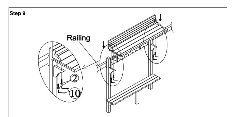
Assemble pre-fixed table from Step 7 and Step 8 together by using Long bolts (2) and Allen key (10) as shown in picture.
