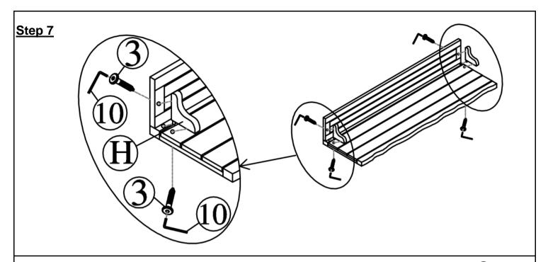
Assembly Upper Support Wings (H) to finish part in Step 6 by using Long Screws ( $\widehat{3}$ ) and Allen Key ( $\widehat{10}$ ) as shown in picture .
