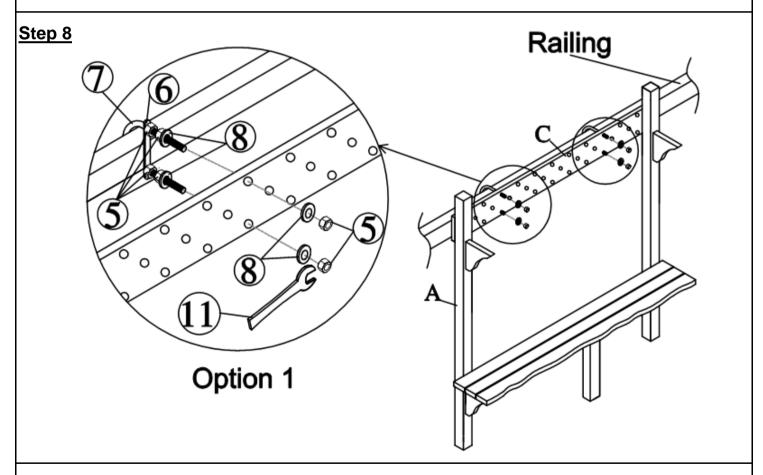
With assistance from your adult partner, stand pre-fixed table in Step 5, right side up. Attach the Table Support Bar (C) to your balcony (railing) by using Horseshoe Bolt (7), Plate (6), Washer, Nut (5) and Spanner (11) as shown in picture.
