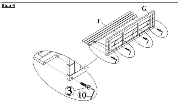
Assembly the Table Top ( G ) to the Back Panel ( F ) by using Allen Key ((10)) to tighten the Long Screws ((3)) in.
