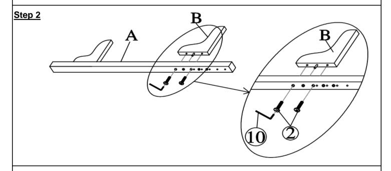
Customer need to check the railing height, matching to table height, before assembly of Lower Support Wing (B).
