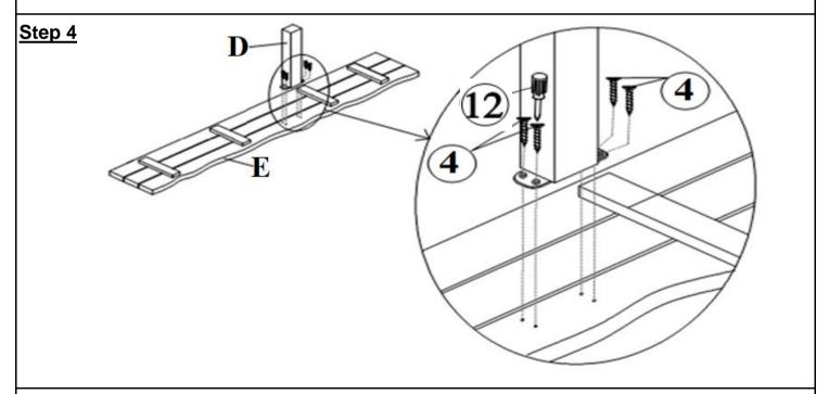
Using Screw Driver ((12)) and Screws ((4)) to assemble the Short Leg (D) to the Footrest Shelf (E) as shown in picture.
