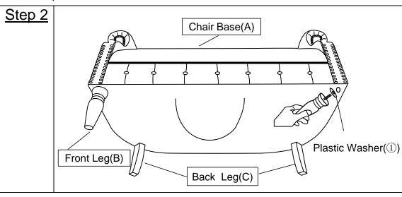
Install the Front Leg(B) into the bottom of the Chair Base(A) by placing the Plastic Washer(①) onto the threaded stem.
