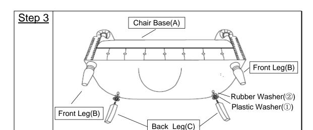
Install the Back Leg(C) into the bottom of the Chair Base(A) by placing the Plastic Washer(1) and Rubber Washer(2) onto the threaded stem. And then insert the threaded Stem into the threaded Mounting Position at each Corner of the Bottom of the Chair Base(A).
