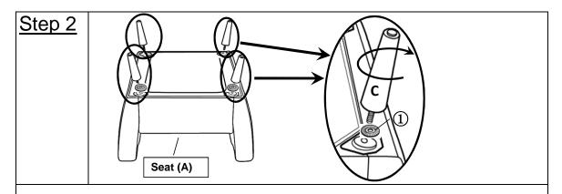
Attach the Legs(C) to Seat(A) with Plastic Washer(1) by turning the legs clockwise as shown.
