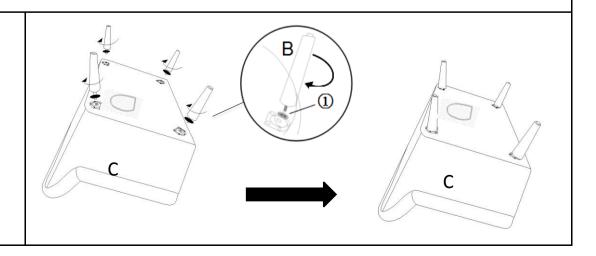
Install the Leg(B)at the bottom of the Sofa by placing one Gasket (①) on the threaded stem.
