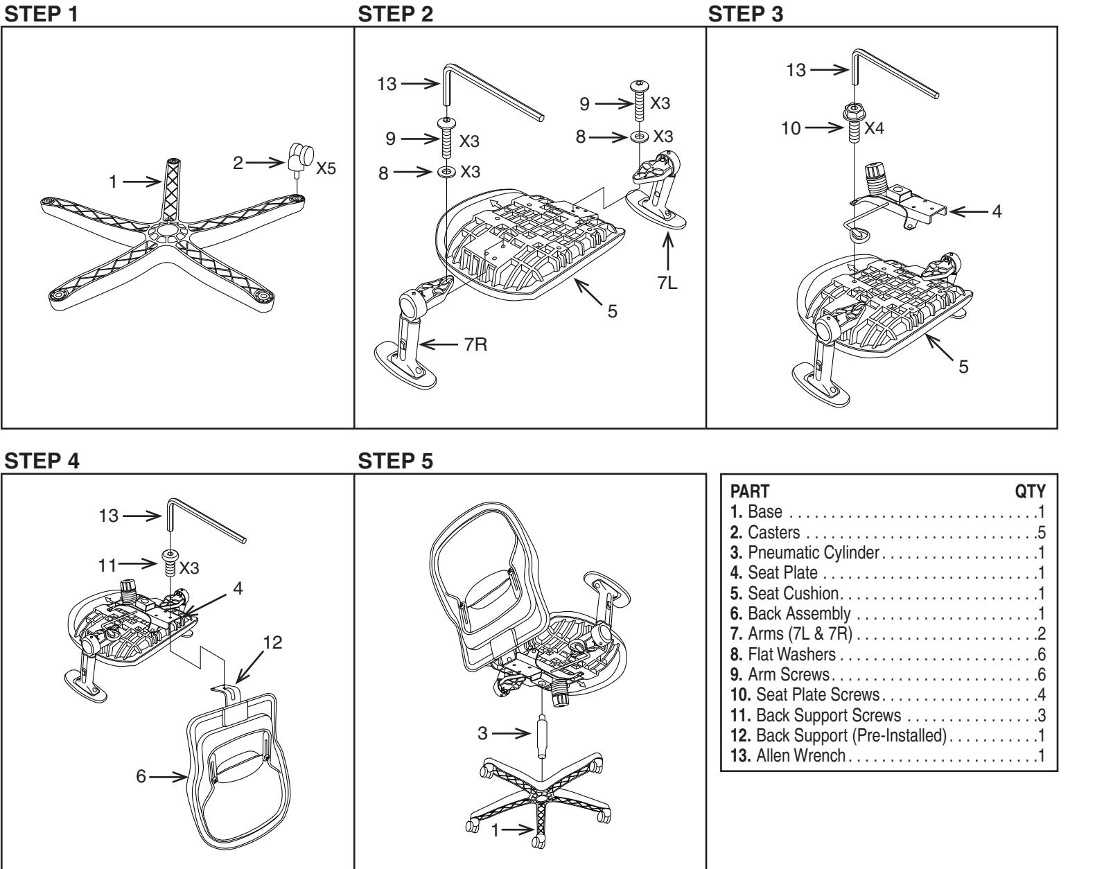
Remove all parts from carton, separate by part numbers indicated on parts list, and verify part quantities.
