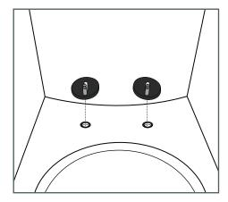
Place seat hardware over where you inserted the threaded rubber pieces.
