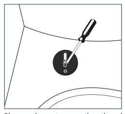
Place washer onto screw then thread screwthrough the seat hardware into the rubber piece. Before you fully screw in hardware, be sure to test position by placing the seat on top and making adjustments if needed.
