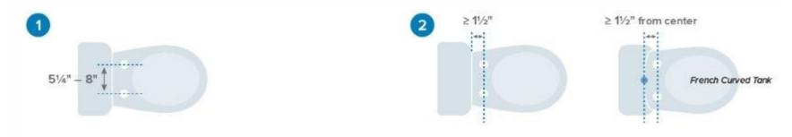
Measure the **distance between the bolt holes**. The space must be between 5½ inches and 8 inches.
