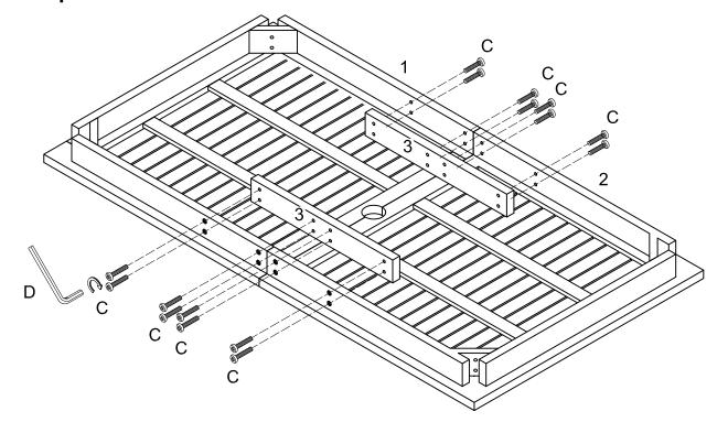
Use wrench (D) to secure part (3) to top frame (1,2) with bolt (C).
