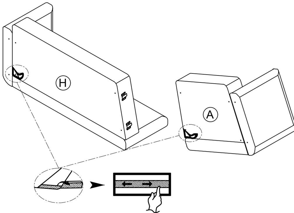
**STEP 4:** Press the fabric flap firmly onto the underside of **Three-Seater Frame (H)** and the **Angled Chair Frame (A)** with Magic tape.
