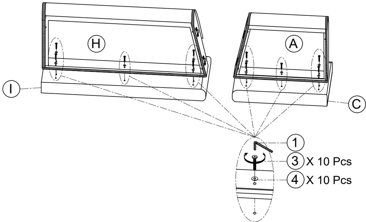
**STEP 2:** Attach the **Three-Seater Frame (H)** to the **Long Backrest (I)**, and attach the **Angled Chair Frame (A)** to the **Short Backrest (C)** using **Bolts (3)** and **Flat washers (4)**. Then tighten securely with an **Allen Wrench (1)**.
