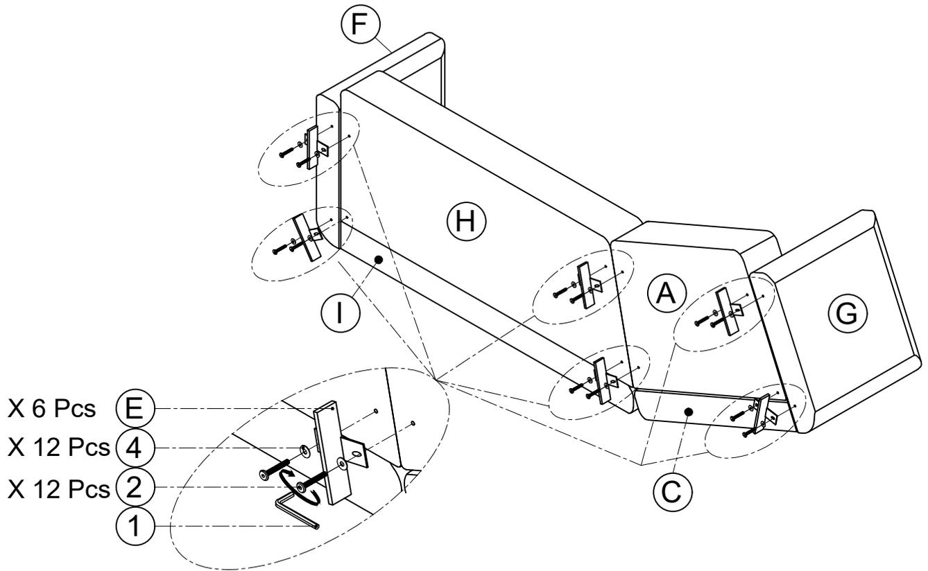
**STEP 6:** Attach the **Legs (E)** to the mounting position on the **Three-Seater Frame (H)** , **Angled Chair Frame (A)** , **Left Arm (F)** and **Right Arm (G)** using **Bolts (2)** and **Flat washers (4)**. Then tighten securely with an **Allen Wrench (1)** .
