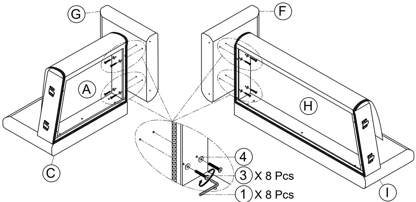
**STEP 3:** Attach the **Three-Seater Frame (H)** to the **Left Arm (F)**, and attach the **Angled Chair Frame (A)** to the **Right Arm (G)** using **Bolts (3)** and **Flat washers (4)**. Then tighten securely with an **Allen Wrench (1)**.
