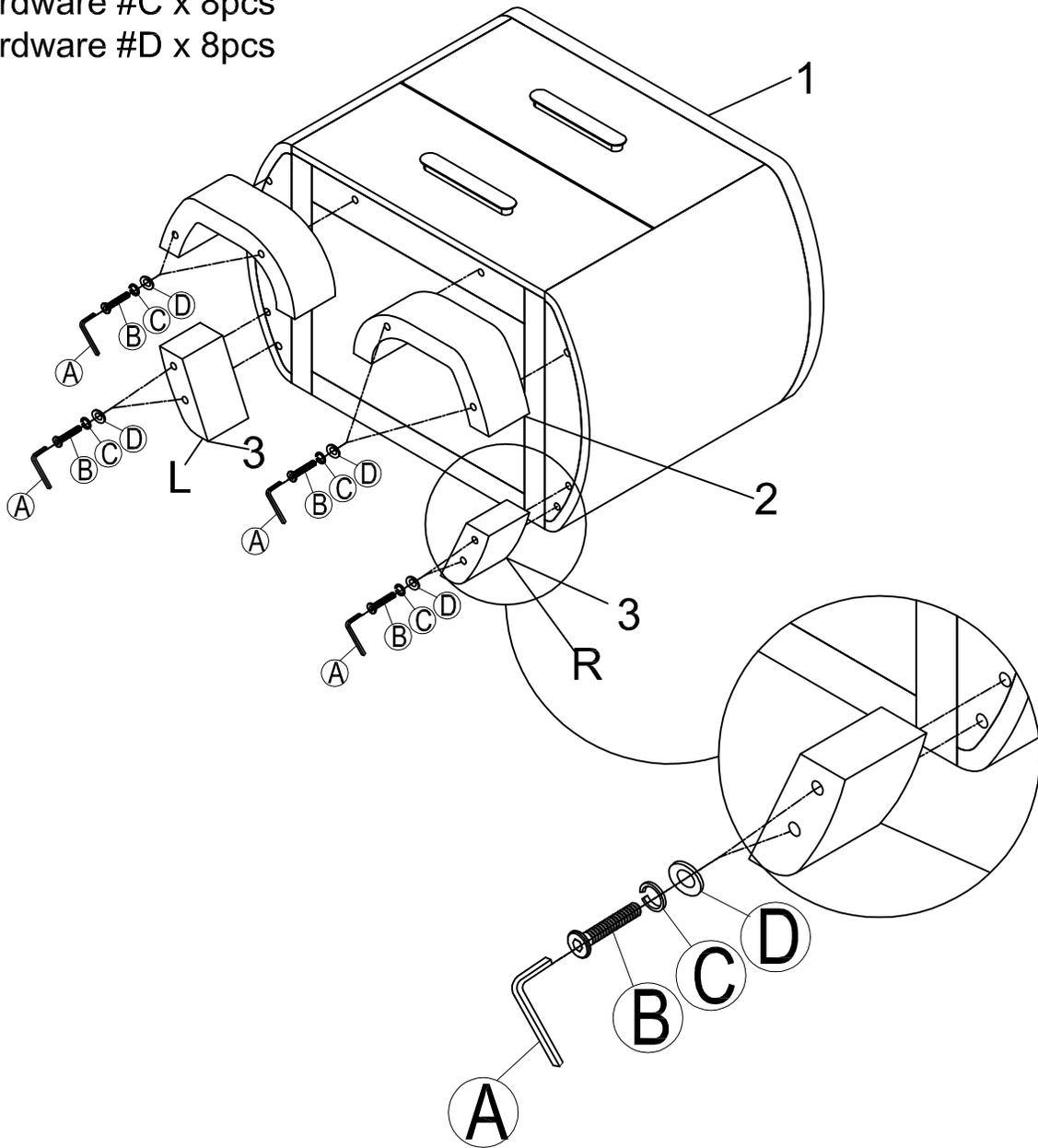
Attach the Front legs(#2 )and Back legs (#3) to the bottom Nightstand (#1) . Secure by using Bolt (#B) with Lock Washer (#C) and Flat washer (#D) Allen wrench(#A).
