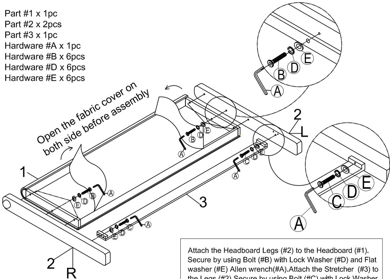
Attach the Headboard Legs (#2) to the Headboard (#1). Secure by using Bolt (#B) with Lock Washer (#D) and Flat washer (#E) Allen wrench(#A). Attach the Stretcher (#3) to the Legs (#2). Secure by using Bolt (#C) with Lock Washer (#D) and Flat washer (#E) Allen wrench(#A).
