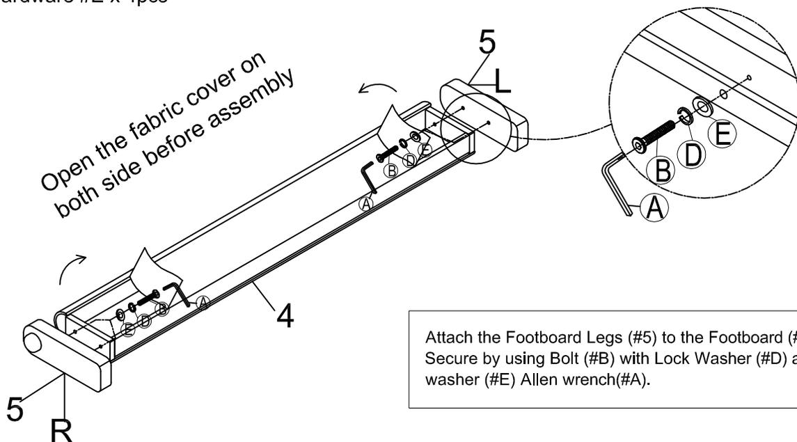
Attach the Footboard Legs (#5) to the Footboard (#4). Secure by using Bolt (#B) with Lock Washer (#D) and Flat washer (#E) Allen wrench(#A).
