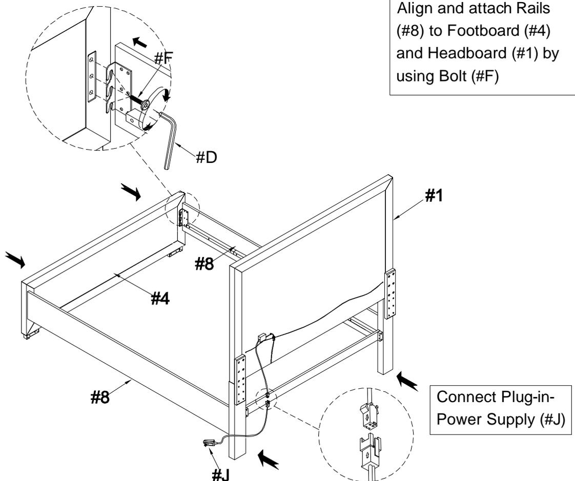
Align and attach Rails (#8) to Footboard (#4) and Headboard (#1) by using Bolt (#F)
