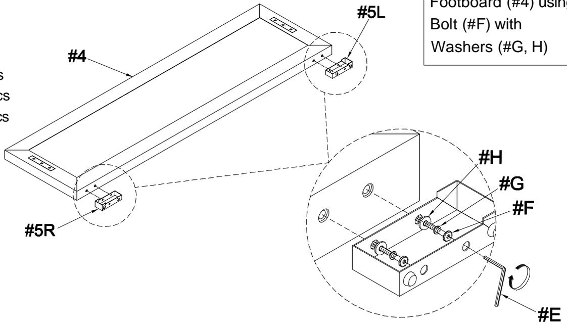
Attach FB Leg (#5) to Footboard (#4) using Bolt (#F) with Washers (#G, H)
