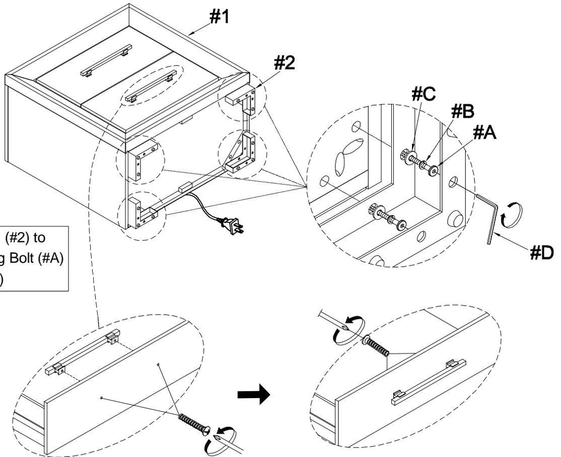
Align and attach Leg (#2) to Nightstand (#1) using Bolt (#A) with Washers (#B, C)
