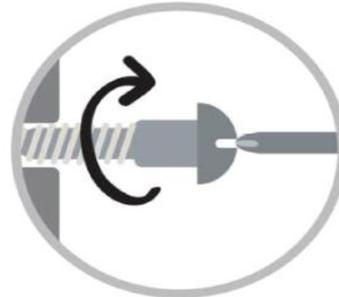
Turn clockwise to tighten and only tighten when step is completed or when instructed to do so.
