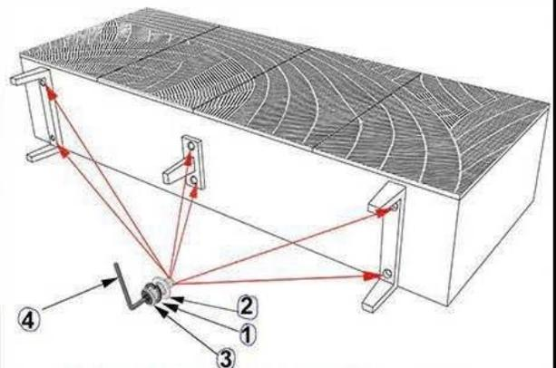
Match holes of legs to holes on bottom before screwing, if holes do not line up, switch the legs
