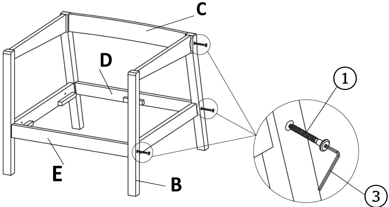
With the help of your adult partner, put the mortises of Right Leg Panel (B) to the tenons of Backrest Panel (C), Back Support Bar (D) and Front Support Bar (E) of the assembled part in Step 2 and then secure by using Screws (①) and Allen Wrench (③) as shown above.
