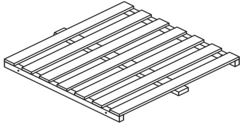
A rectangular panel with a grid of horizontal and vertical slats, used for the seat backrest.             | Seat Panel        | 1 |
