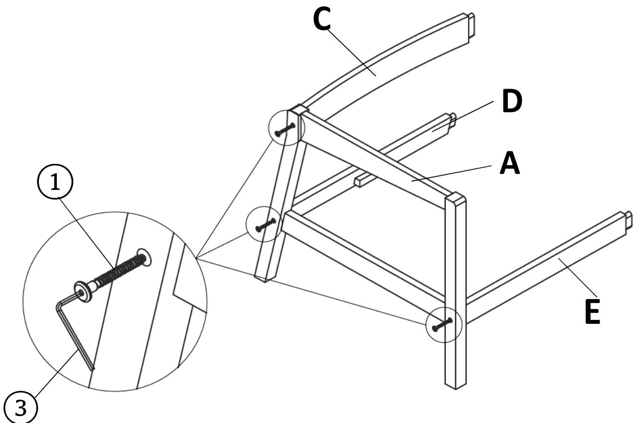
With the help of your adult partner, put the tenons of Backrest Panel (C), Back Support Bar (D) and Front Support Bar (E) to the mortises of Left Leg Panel (A) and then secure by using Screws (①) and Allen Wrench (③) as shown above.
