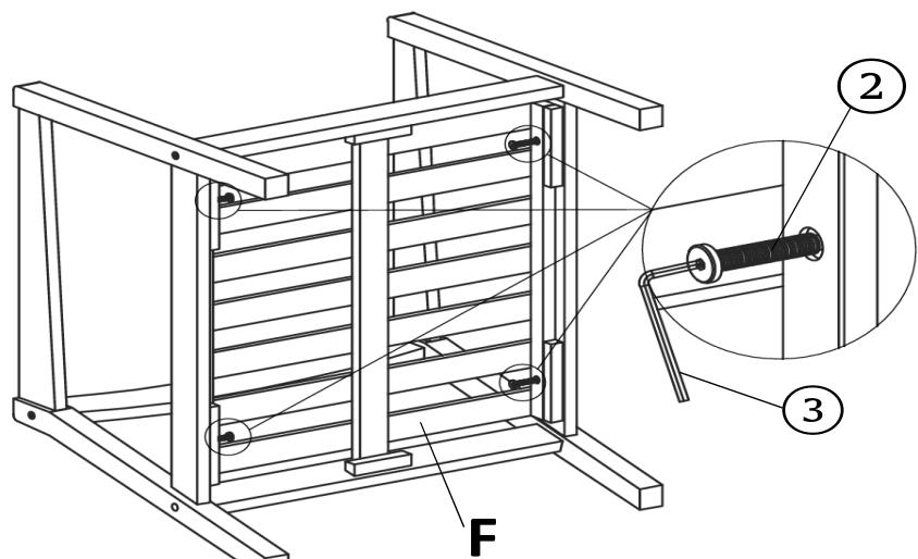
Place the Seat Panel (F) to the assembled part in Step 3 and then turn the above frame back side down and secure the Seat Panel (F) to the Left Leg Panel (A) and Right Leg Panel (B) by using Bolts (2) with Allen Wrench (3) as shown above.
