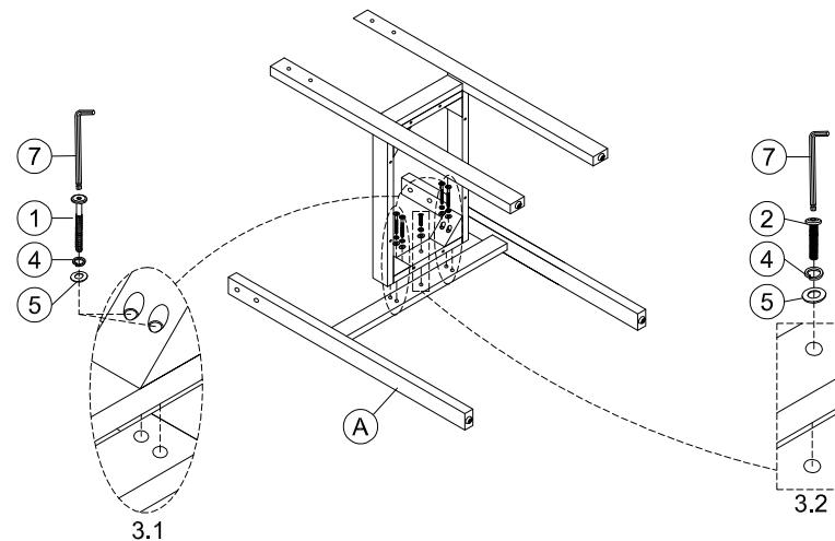
3.1. Assemble the part in Step 3 to the Front chair frame (A) using bolt (1). Spring Washer (4) Flat washer (5) Allenkey (7)
