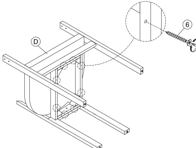
Assemble the Seat Frame With Cushion (D) into the part in Step 4 ,using the Wood screws (6)
