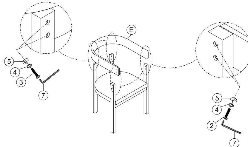
Assemble the Back Frame (E), into the part in step 5,using the bolt (2) for the front and (3) for the back , Spring Washer (4) flat washer (5), Allen key (7).
