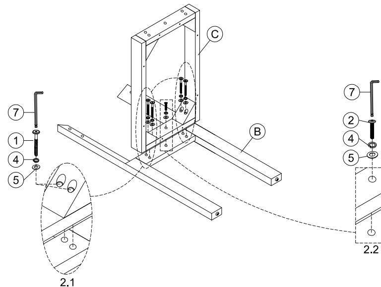
2.1. Assemble the Upper chair frame (C) to the Back chair frame (B) using blot (1). Spring Washer (4) Flat washer (5) Allenkey (7)
