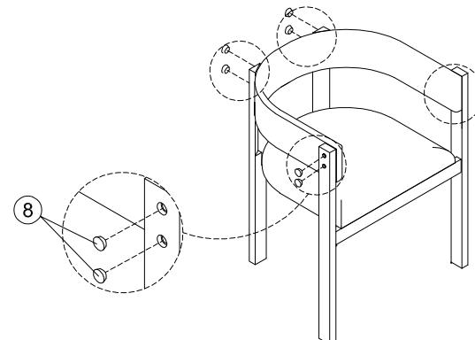
Close the Wooden Plugs (8) tightly to the previous bolt catch hole
