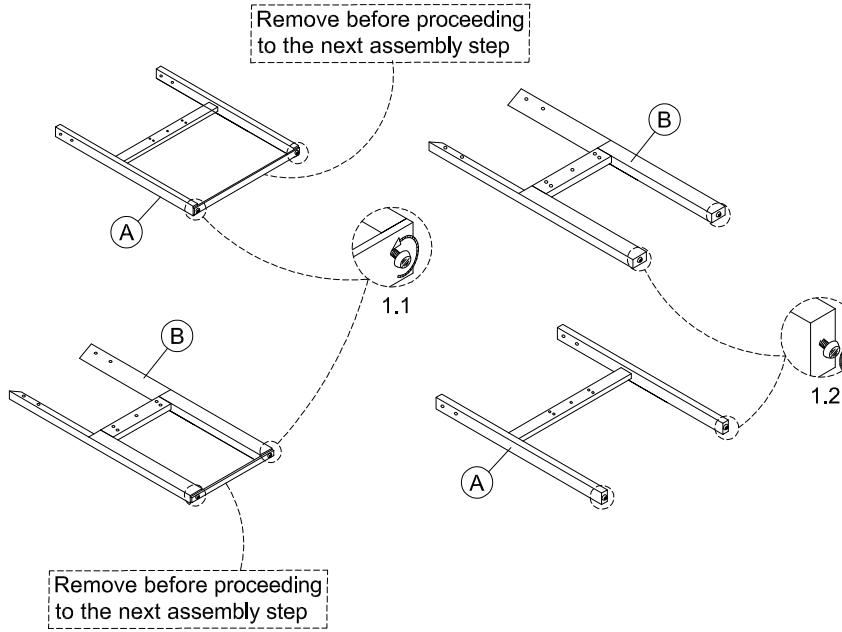
1.1. Remove the support bar pre-assembled on the Front chair frame (A) and the Back chair frame (B) by turning the Leveler counterclockwise.
