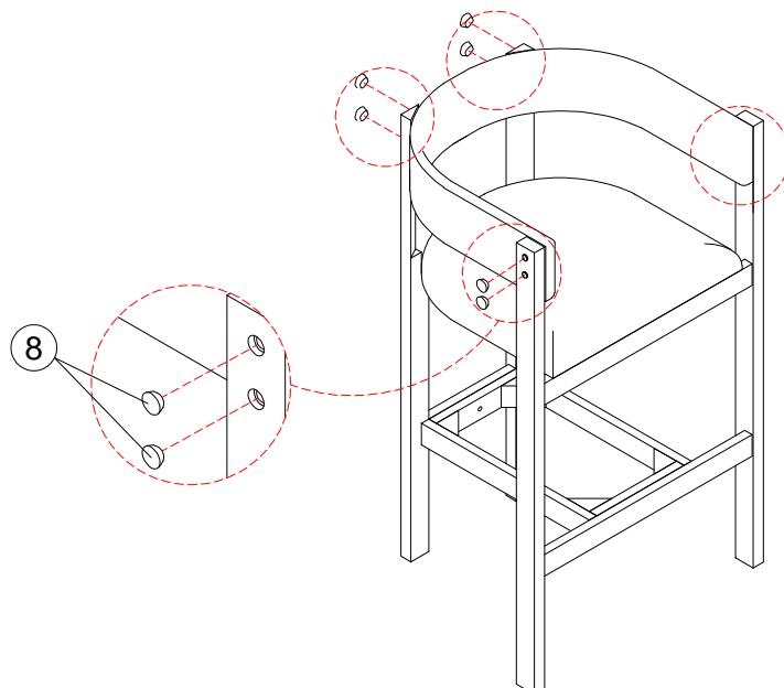
Close the Wooden Plugs (8) tightly to the previous bolt catch hole
