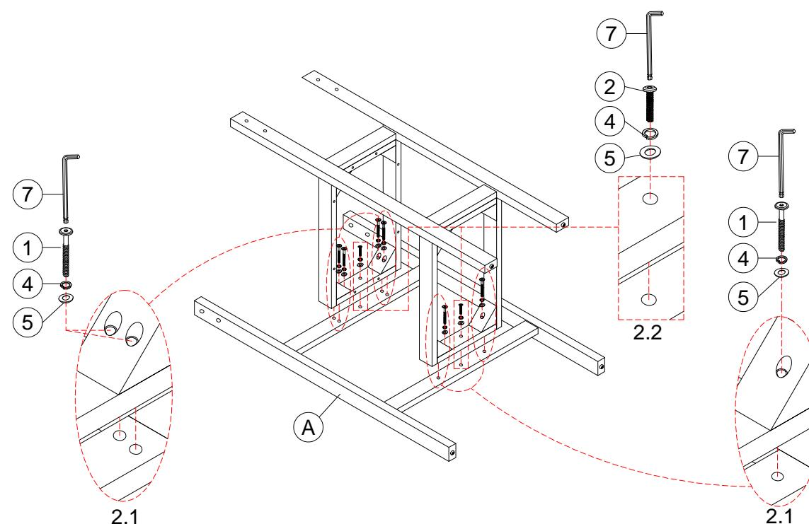
2.1. Assemble the part in Step 2 to the Front chair frame (A) using blot (1). Spring Washer (4) Flat washer (5)
