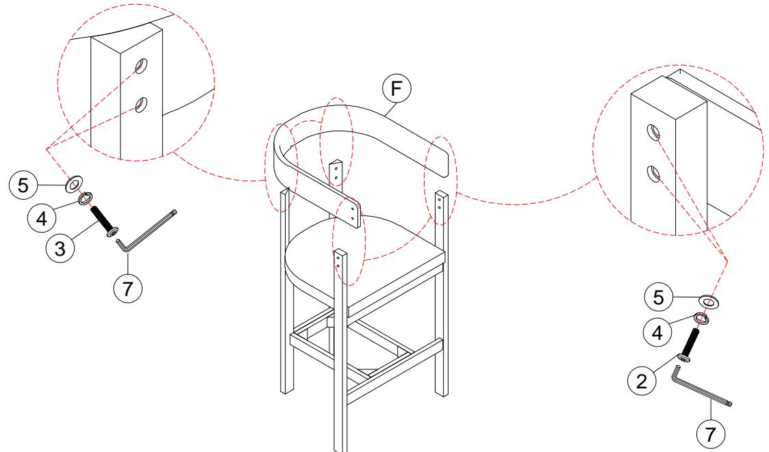
Assemble the Back Frame (F), into the part in step (4),using the bolt (2) for the front and (3) for the back , Spring Washer (4) flat washer (5), Allen key (7).
