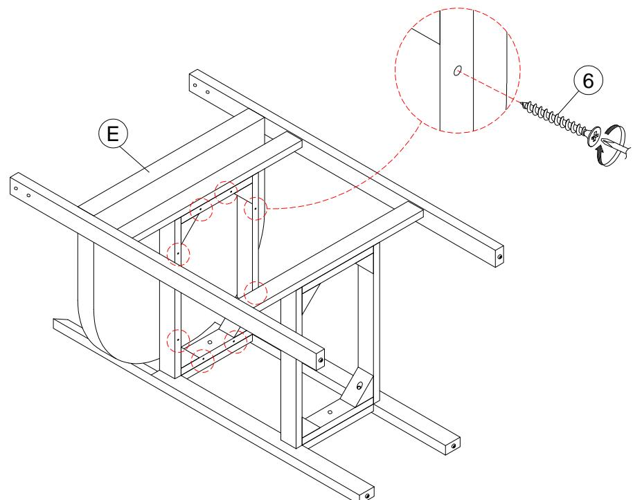
Assemble the Seat Frame With Cushion (E) into the part in Step 3 ,using the Wood screws (6)
