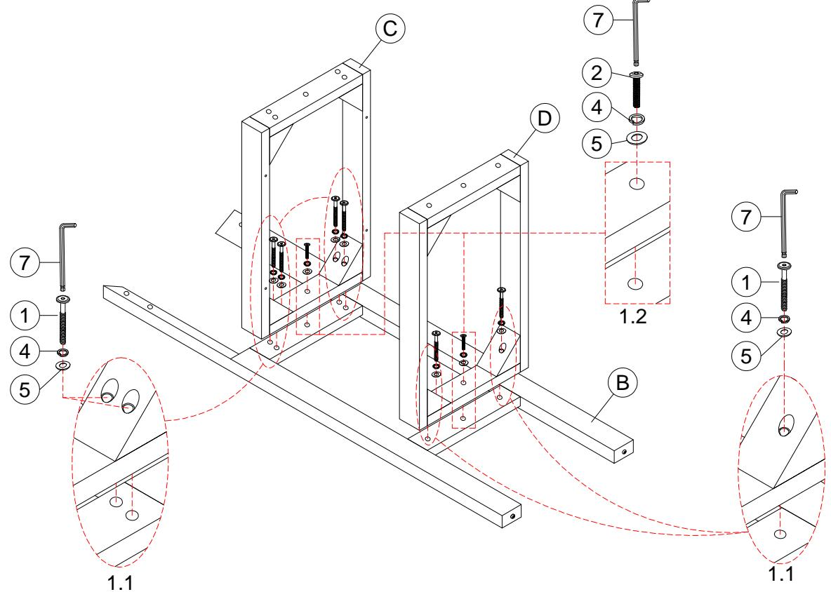
1.1. Assemble the Upper chair frame (C),Lower chair frame (D) to the Back chair frame (B) using blot (1).
