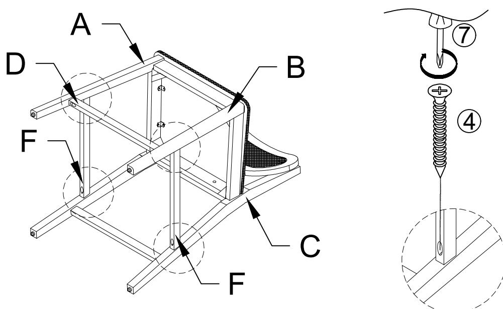
Place the Tie Rod (F) onto the Backrest (C), and the Tie Rod (Front) (D) into the Front Leg (Left) (A) and the Front Leg (Right) (B), using the Screwdriver ( 7 ) and Screws ( 4 ) . Tighten the Screws, and bolts.
