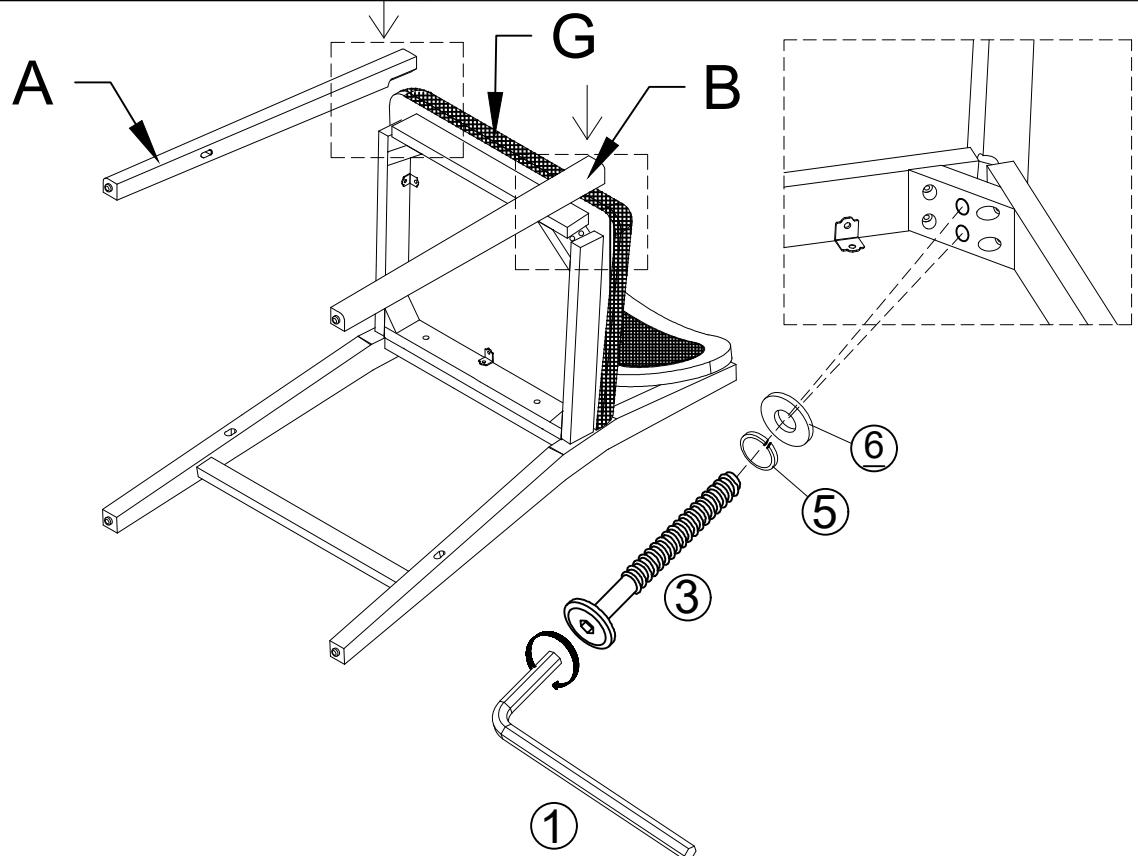
Place the Front Leg (Left) (A) and the Front Leg (Right) (B) onto the Seat Cushion (G), using the Allen Wrench ( 1 ), Bolts ( 3 ), Spring Washer ( 5 ), Flat Washer ( 6 ) . Tighten the Bolts 80%.
