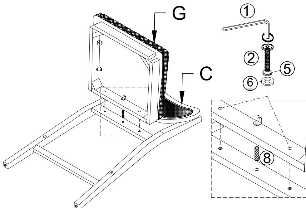
Place the Seat Cushion (G) onto the Backrest (C) using the Allen Wrench (1), Bolts (2), Spring Washer (5), Flat Washer (6), Wood dowel (8) as pictured above. Tighten the Bolts 80%.
