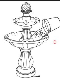
Fill the larger basin(D) with clean water, making sure the pump (G) is fully submerged.
