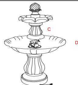
Make sure the threaded poles on the larger basin(D) are inserted securely into the connector(C)
