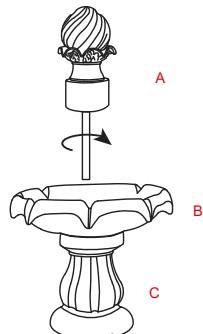
Route the pre-assembled water hose on the top (A) through the basin (B) and connector (C), turning it counterclockwise until the triangle marks line up.
