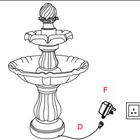
Finally, connect the cord of pump (G) to transformer(F), then plug the transformer into power supply.
