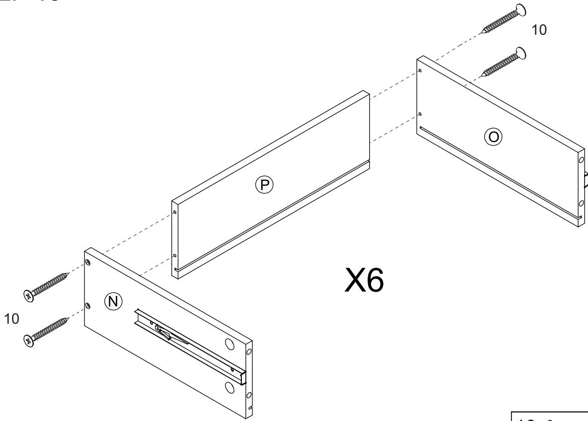
Attach Drawer Left Panel (N) and Drawer Right Panel (O) to the Drawer Back Panel (P) using Screw (10) with Screwdriver (Not provided).
