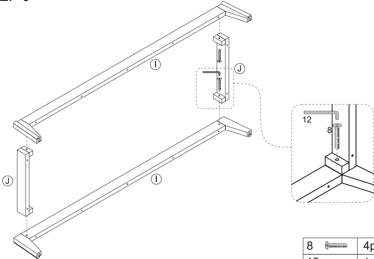
Attach Support Bar (J) to Leg Panel (I) using Bolt (8) with Allen Wrench (12).
