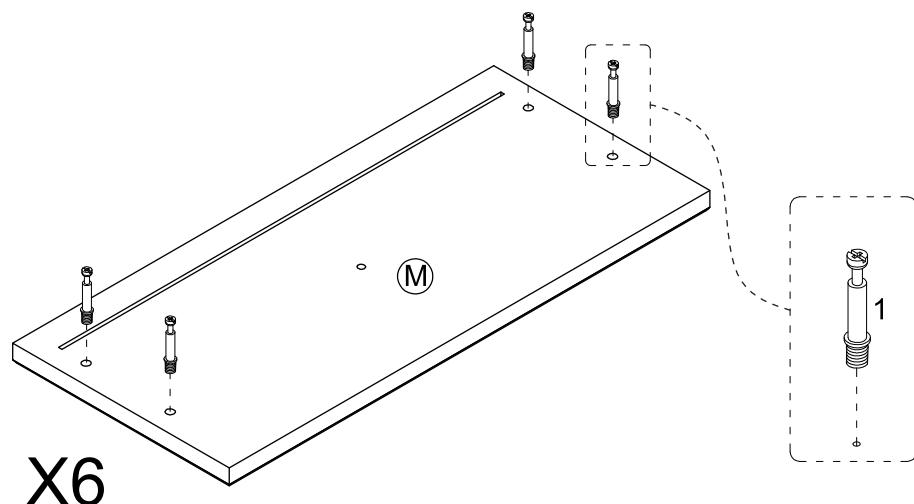
Insert Three in one bolt (①) into drilled holes on the Drawer Front Panel (M) with Screwdriver (Not provided).
