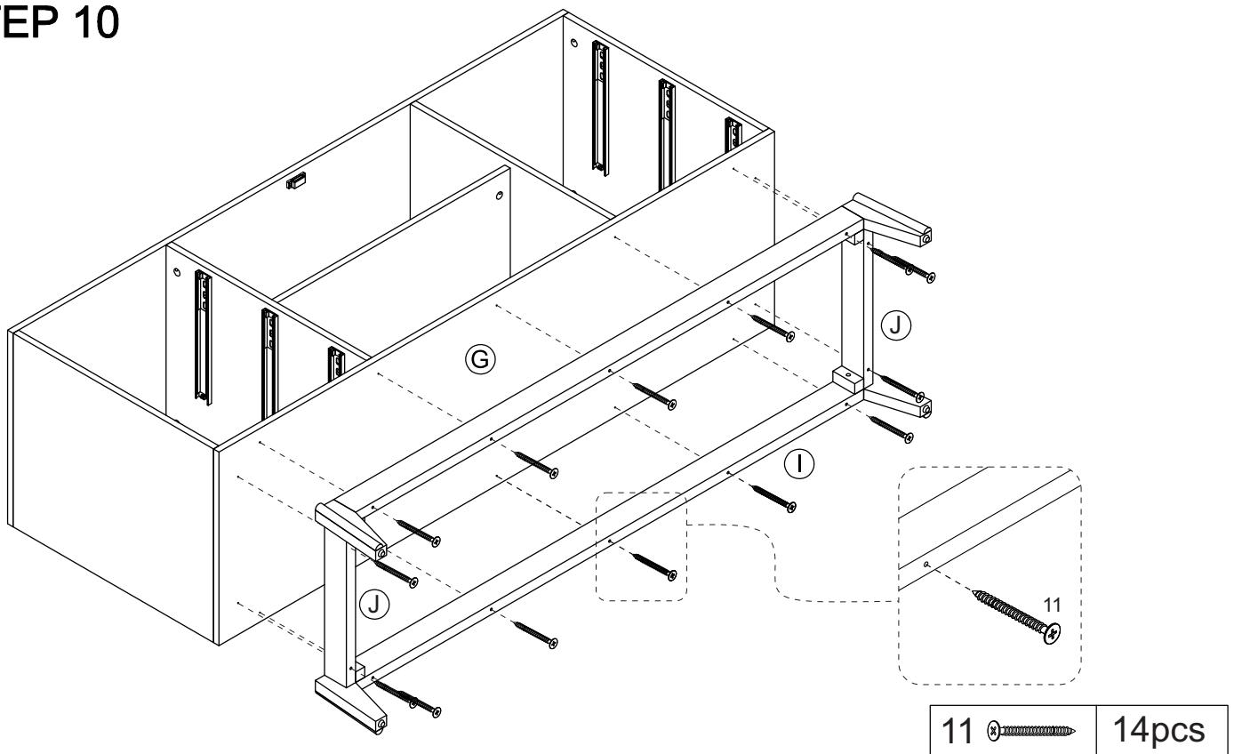
Attach Leg Panel (I) and Support Bar (J) to Bottom Panel (G) using Screw (11) with Screwdriver (Not provided).
