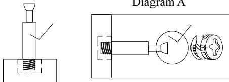
Insert Cam Ball into hole as shown in diagram A.
