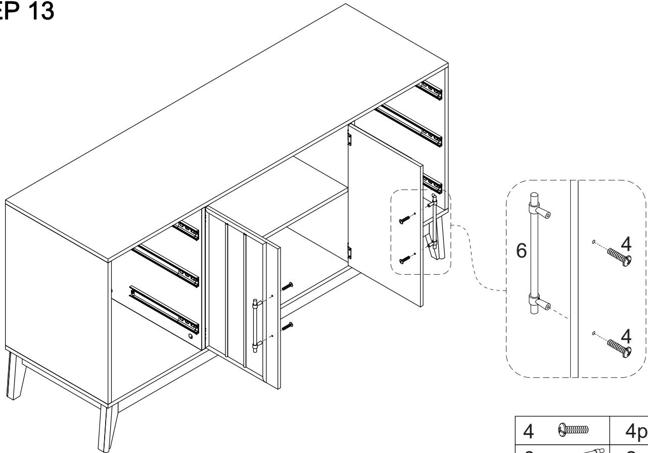
Attach Handle (⑥) to the Door using Bolt (④) with Screwdriver (Not provided).
