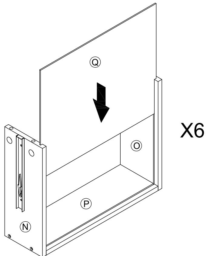
Attach Drawer Back Panel (Q) to the Drawer Left Panel (N), Drawer Right Panel (O) and Drawer Back Panel (P).
