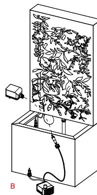
Connect and insert the pipe into the Pump(B).
