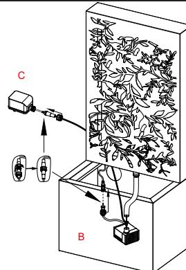
Connect the transformer(C) and light wires to the pump(B) showed as above.
