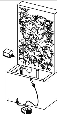
Place the fountain on a level surface away from areas where it is likely to get clogged with leaves and make sure that the cable will reach the socket and open the back door(anticlockwise).
