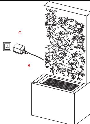
Plug the Pump(B) and Transformer(C) in the socket showed as above.
