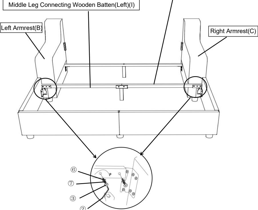
Install the Middle Leg Connecting Wooden Batten(I ) and(J) on the Left Armrest(B) and Right Armrest(C) by using Bolt (③), Spring Washer(⑦) ,Flat Washer(⑥) and Allen Wrench(②),turning clockwise until tight.
