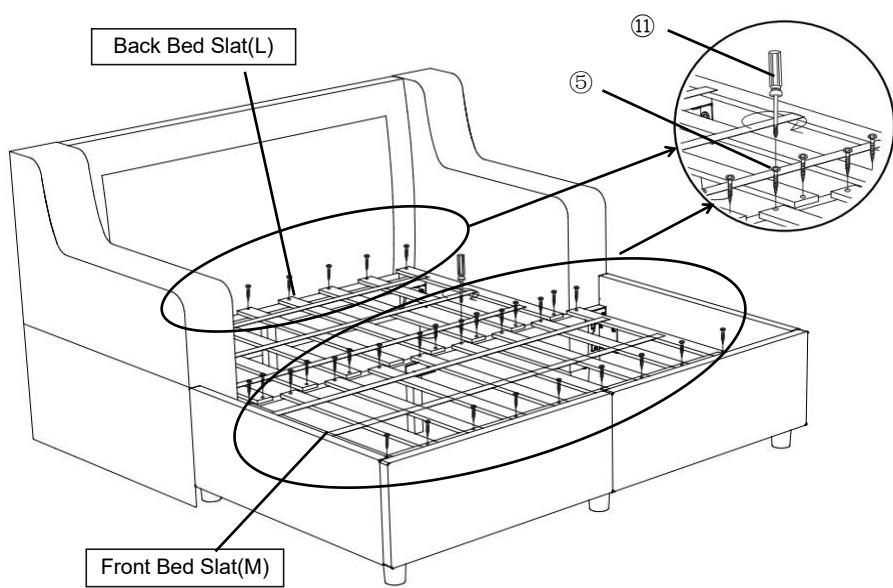
Use a screwdriver(⑪) to fix the screw(⑤) and the Back Bed Slat(L) and Front Bed Slat(M) to the slat. A total of 33 screws are needed.
