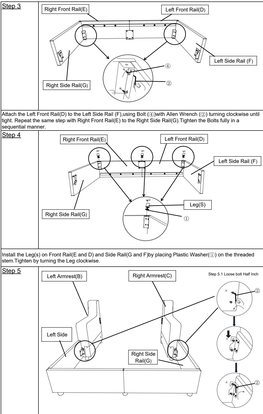
Step5.1. Loose the bolts Half Inch by Allen Wrench(②).
