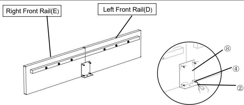
Connect Right Front Rail(E) and Left Front Rail(D) by using Iron Connecting Plate(⑧), Bolts(④) with Allen Wrench(②) turning clockwise until tight.
