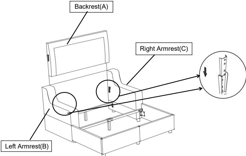
Slide the Tapered Connectors on the Backrest(A) into the Tapered Connectors on the Left Armrest(B) as shown in the picture. Repeat the same steps with the Right Armrest(C).
