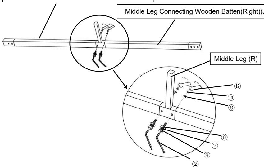
Assemble the Middle Leg(R) on two Middle Leg Connecting Wooden Batten(I ) and(J) by using Bolt(③) ,Spring Washer(⑦),Flat Washer(⑥) and Allen Wrench(②),Nut(⑩),Flat Washer(⑥),and Spanner(⑫) turning clockwise until tight.
