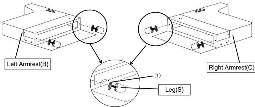
Step 1. Install the Leg(S) at the bottom of Left Armrest(B) and Right Armrest(C) by placing Plastic Washer(①) on the threaded stem. Tighten by turning the Leg clockwise.
