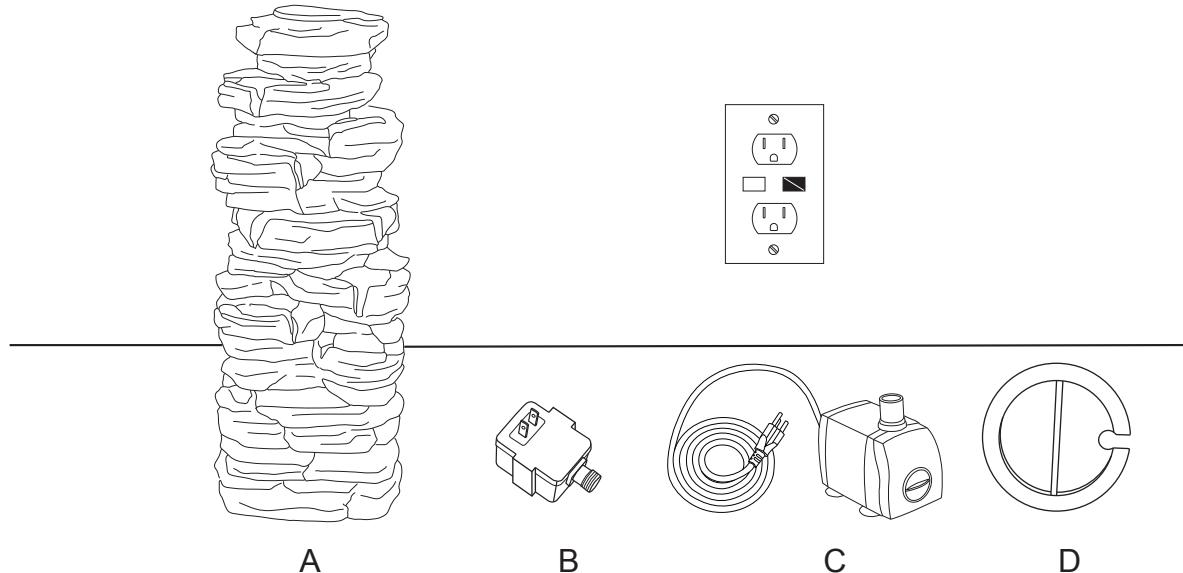
**STEP 2** Connect the pre-installed light cable inside Fountain (A) to Power Plug(B). Tighten the connector by twisting clockwise.
