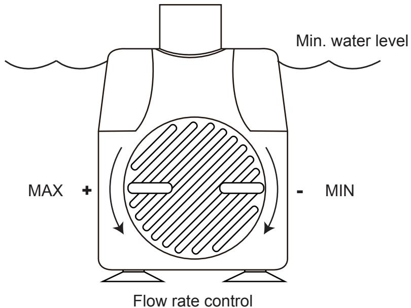
**STEP 4** Connect the pre-installed water hose inside Fountain (A) to Pump (C) through the back opening. Position Pump (C) into fountain reservoir.
