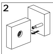
2: Join the two pieces by sliding the Cam Bolt into the hole on the side of the piece.
