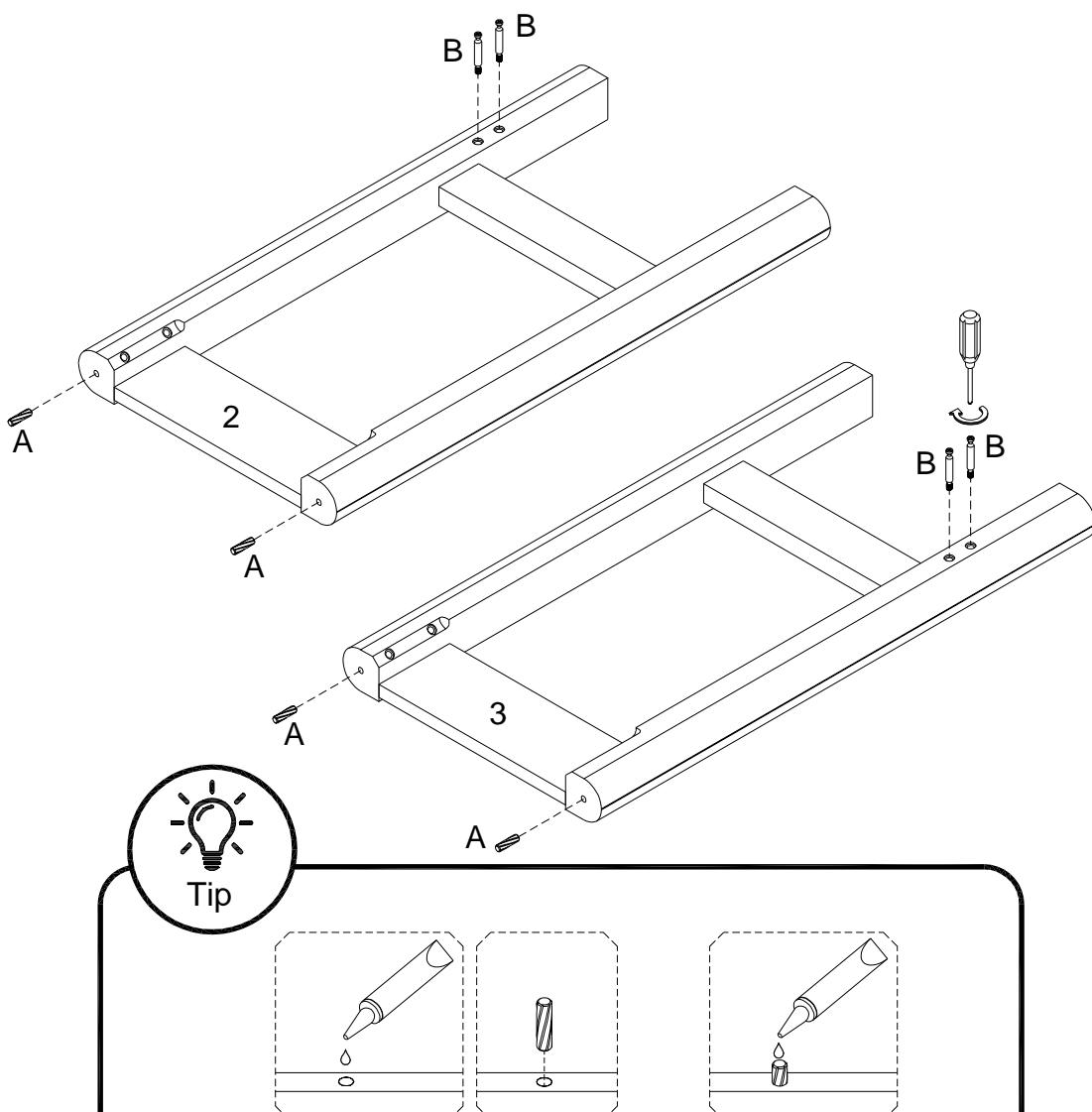
1: The provided glue is to secure wood dowels in place. When first inserting dowels, locate the appropriate hole for the dowel, place a small amount of glue in the hole and insert the dowel. Wipe away excess glue immediately.
