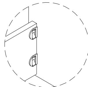
2. Once the pin is inserted correctly, flip the metal lever in the opposite direction to ensure the panels are firmly locked together.
