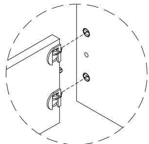
1. Make sure the quick assembly drawer pin is aligned with the corresponding hole.
