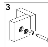
3: Insert the Cam Lock Nut and securely tighten it with a screwdriver.
