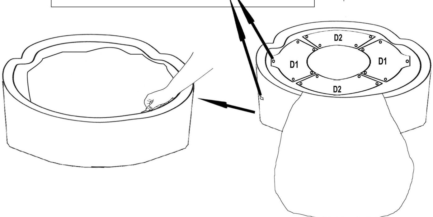
Step 2: Attach the 16 screws to the iron frame and fasten them firmly into the designated screw holes on the wooden panels. Ensure the iron frame is placed flat on the ground as illustrated in the accompanying image or instructional video.
