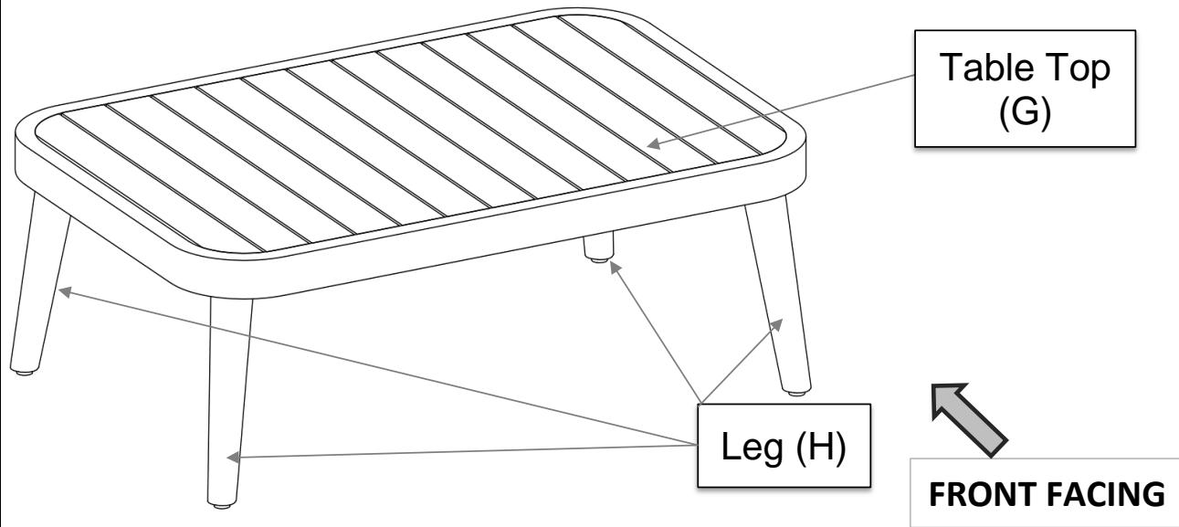
This Table has multiple parts and may require up to 10 minutes to assemble. To give you an overview of the Table, the above picture is to help you put the various parts into perspective. Please read through the instructions here below to familiarise yourself with the parts and steps before assembly.
