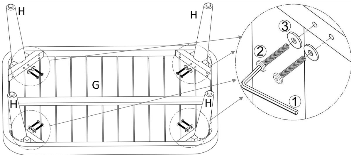
With assistance from your adult partner, attach Legs (H) to Table Top (G) by using Bolts (②) and Washers (③) with Allen Wrench (①) as shown above. **DO NOT** fully tighten the Bolts.
