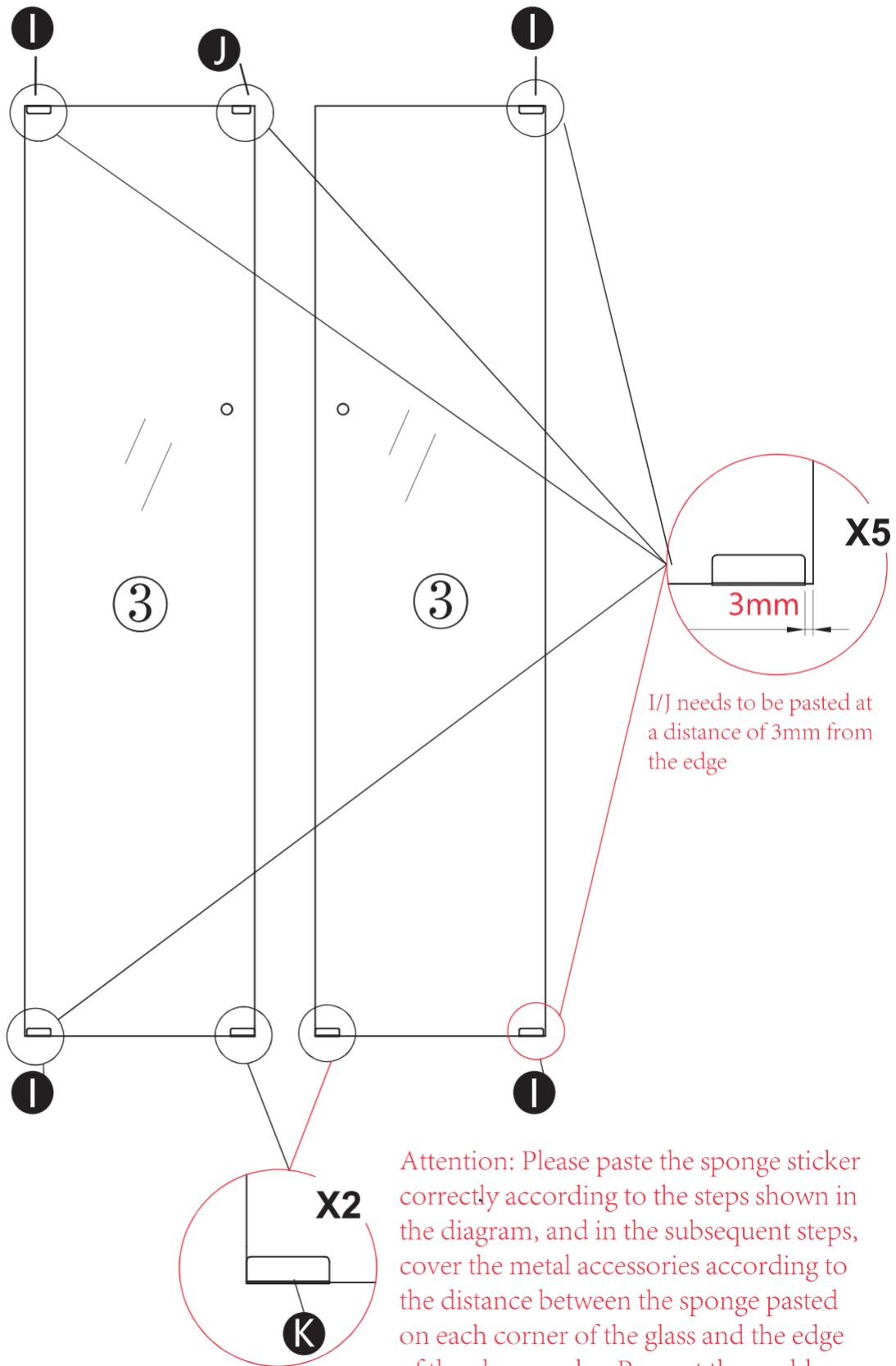
Attention: Please paste the sponge sticker correctly according to the steps shown in the diagram, and in the subsequent steps, cover the metal accessories according to the distance between the sponge pasted on each corner of the glass and the edge of the glass nearby. Prevent the problem of glass doors not being able to close in the future.
