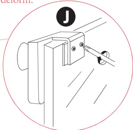
Point: During the installation process, it is necessary to continuously adjust with a key, align the position, and then tighten the screws
