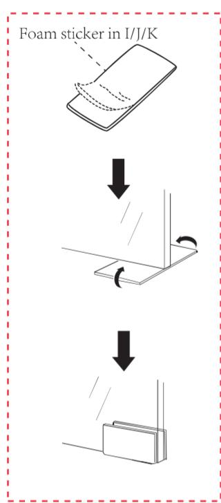
When pasting, the front and back length of foam should be as consistent as possible.
