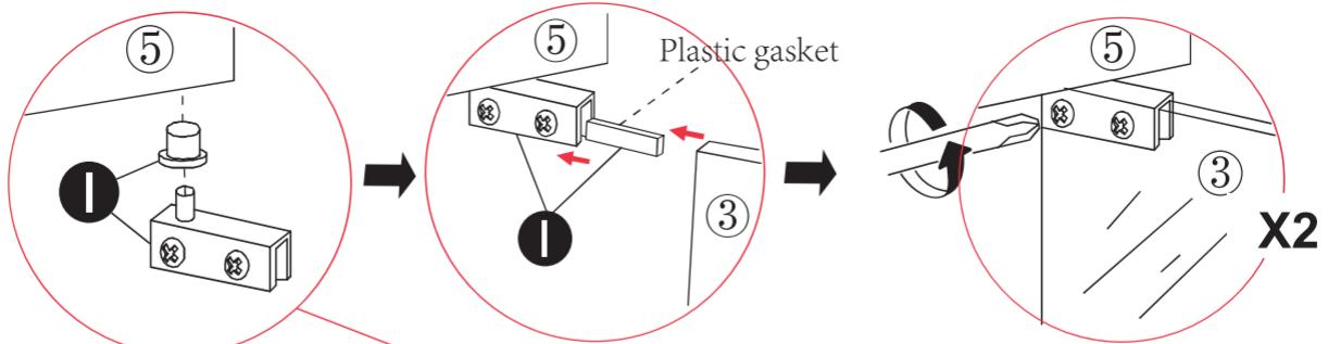
Attention: The side with screws faces inside the cabinet. A plastic sheet is placed between the sponge and nut to prevent the glass from breaking.
