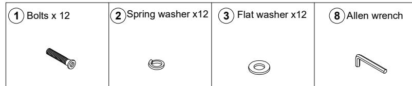
Attach the side rail (C) to the headboard (A/B) and the footboard (D) using bolts (1), spring washers (2) and Flat washers (3) with Allen wrench (8)
