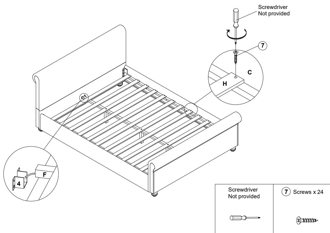
Attach the completed slats (H), Middle support bar (F), Middle support legs(G) to the side rail (C) using screws (7), by screwdriver ( Not provided )
