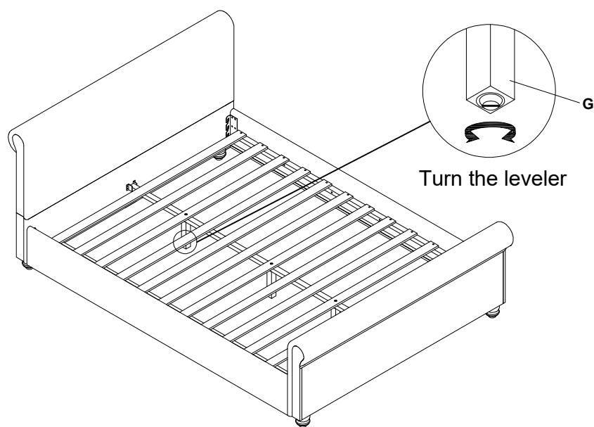
For the middle support legs (G), turn the leveler in to retract and out to extend.
