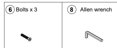
Attach the middle support legs (G) to middle support bar (F) and the slats (H) using bolts (6), with allen wrench (8).
