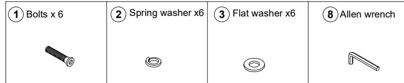
Attach the headboard below (B) to the headboard (A) using bolts (1), spring washers (2) and Flat washers (3) with allen wrench (8)
