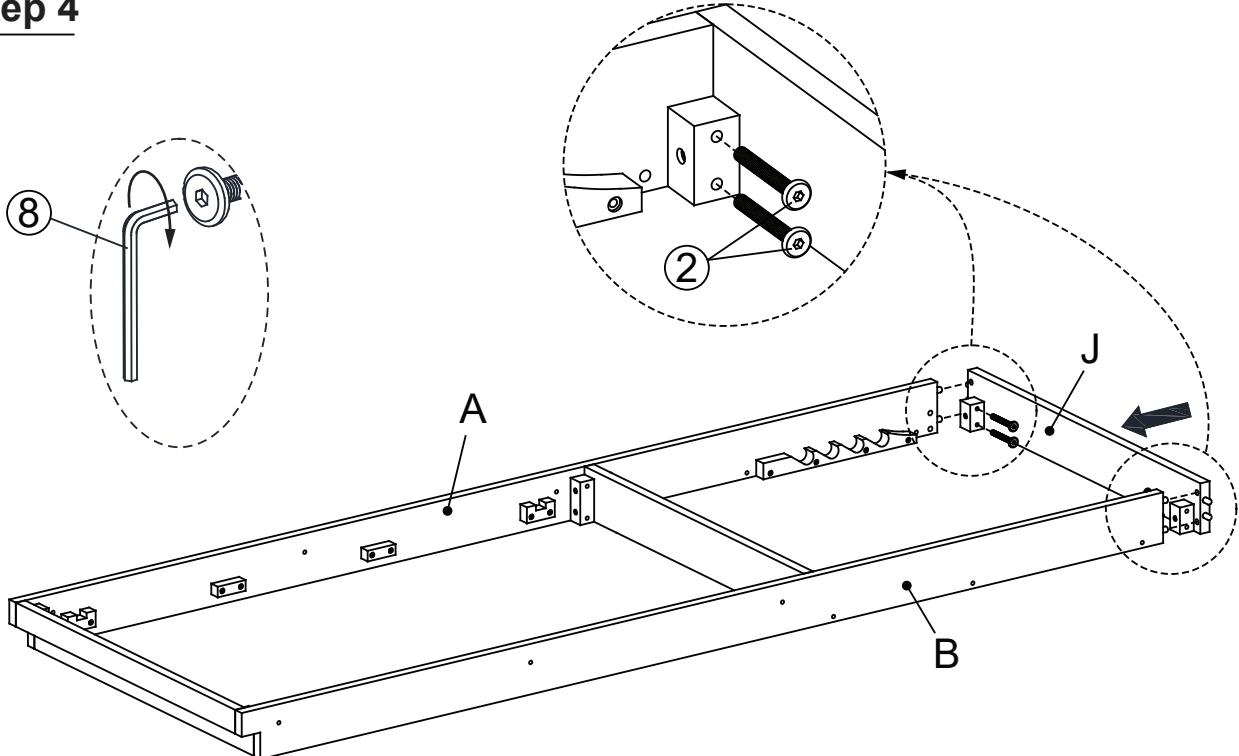
Attach the Head Support Bar (J) to the Left Side Bed Bar (A) and the Right Side Bed Bar (B) by using Bolts (2) and Allen Wrench (8).
