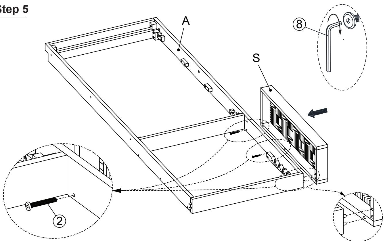
From Step 4, attach the Left Armrest Cluster (S) to the Left Side Bed Bar (A) by using Bolts (2) and Allen Wrench (8).
