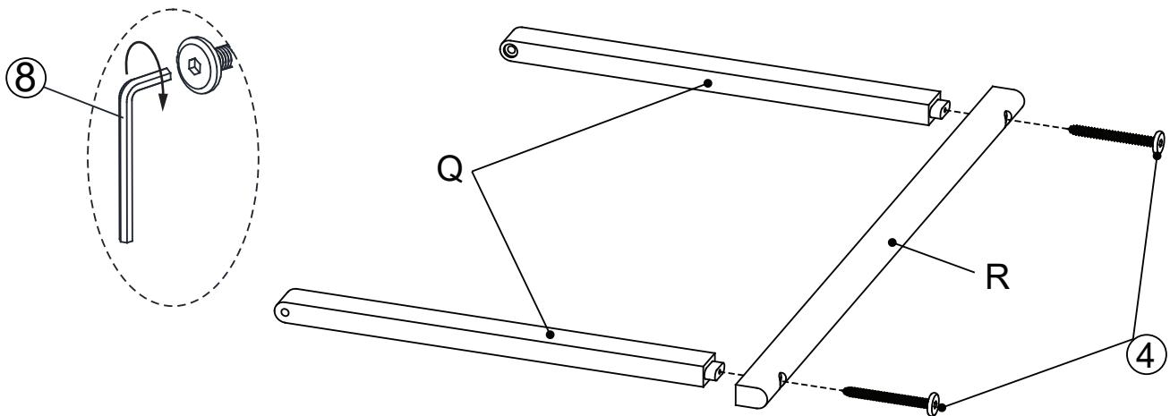
Place the Vertical Bar (Q) and Horizontal Bar (R) on the clean, non-marring surface. Attach the tenon of Vertical Bar (Q) to the Horizontal Bar (R) by using Screws (4) and Allen Wrench (8).
