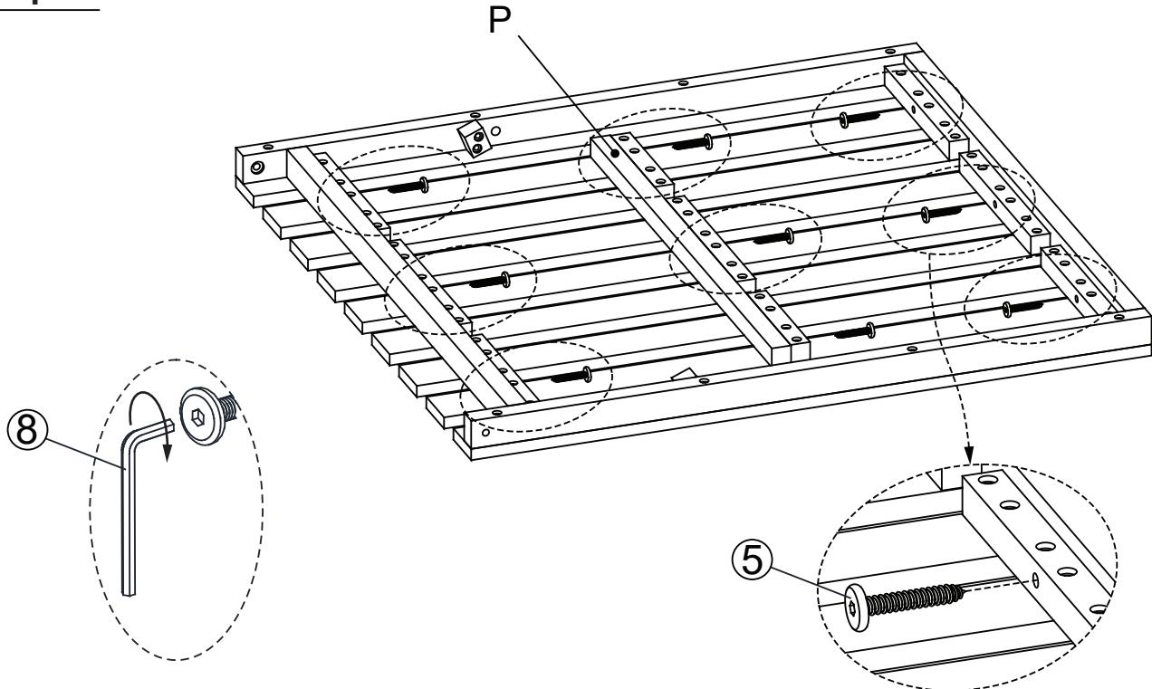
From step 9, attach the Middle Backrest Support Bar (P) to the assembled part in Step 8 by using Screws (5) and Allen Wrench (8).
