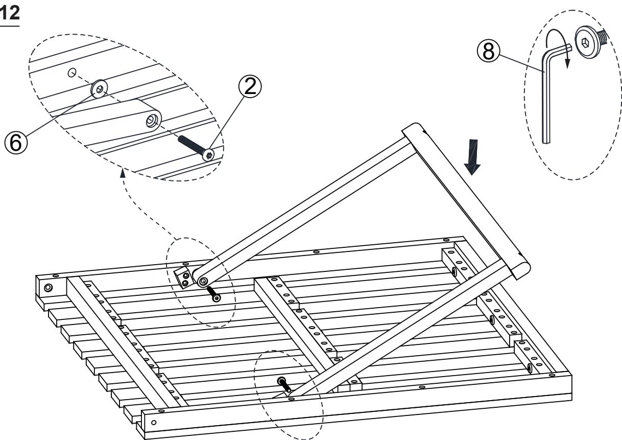
Attach the assembled part in Step 10 to the assembled part in Step 11 by using the Bolts (2), Washer Plastic (6), and Allen Wrench (8).
