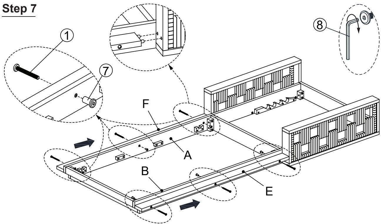
Turn the assembled part in Step 6 to the right side as shown above. Attach the Right Support Bar (E) to the Right Side Bed Bar (B) and Left Support Bar (F) to the Left Side Bed Bar (A) by using Bolts (1), Horizontal Nut (7) and Allen Wrench (8), as shown above.
