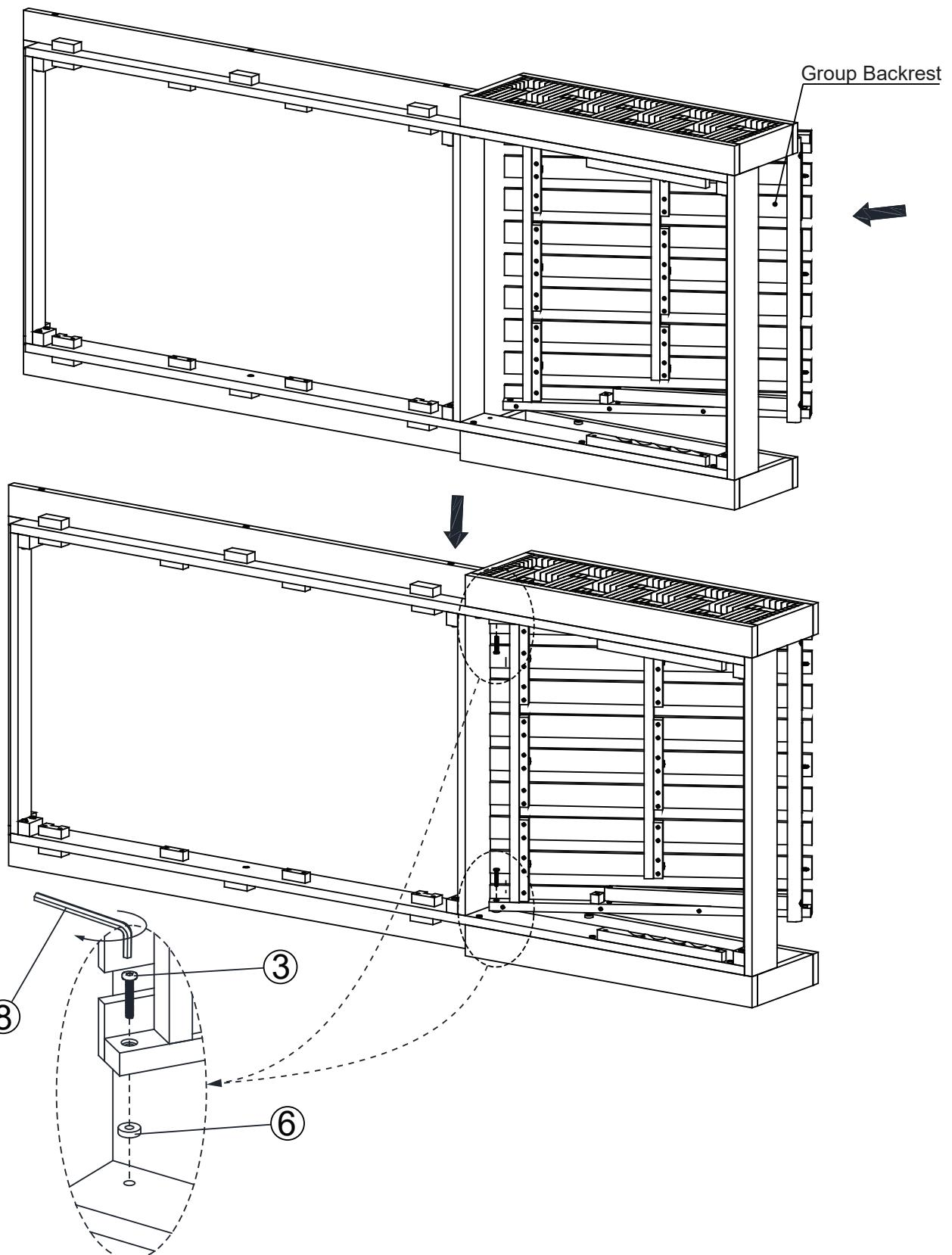
With the help of your adult partners, flip up the assembled part in step 7 (left side-bottom), then attach the assembled part in step 12 to the assembled part in step 7 by using Bolts (③), Washer Plastics (⑥), and Allen Wrench (⑧). Note: DO NOT fully tighten the Bolts at this time.
