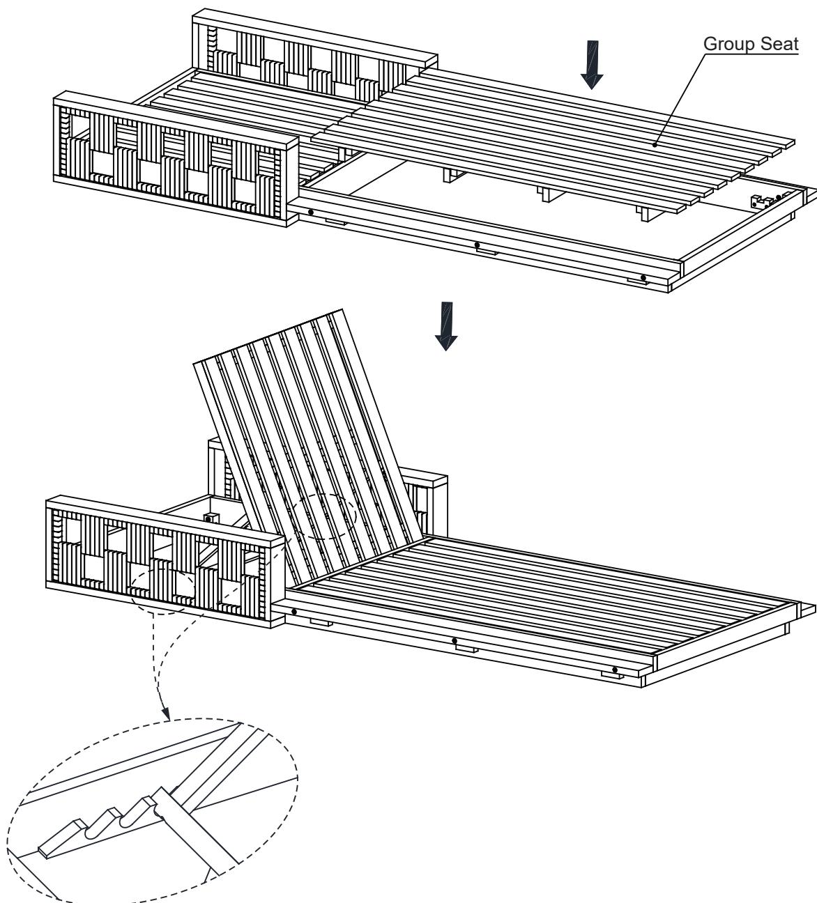
With the help of your adult partners, place the assembled part in Step 13 on the clean, non-marring surface. Attach the assembled part in Step 10 to the assembled part in Step 13 as shown above.
