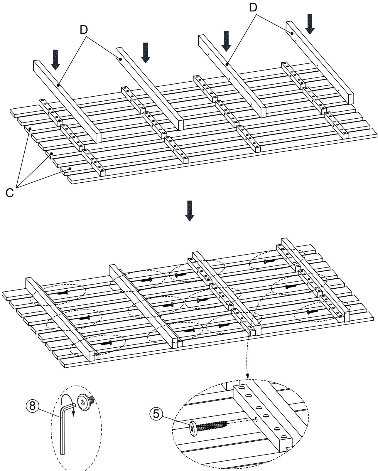
Place the Seat Frame on a clean, non-marring surface. Attach all the Support Bar (D) to the Seat Frame (C) by using Screws (5), Allen Wrench (8) as shown above.
