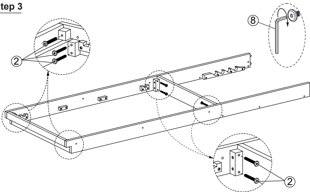
Attach the parts by using Bolts (2) and Allen Wrench (8) as shown above.
