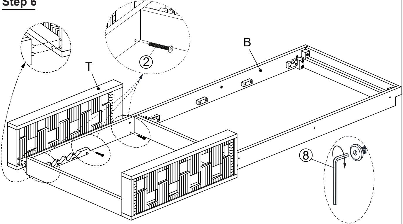
Turn the assembled part in Step 5 to the left side as shown above. Attach the Right Armrest Cluster (T) to the Right Side Bed Bar (B) by using Bolts (2) and Allen Wrench (8).
