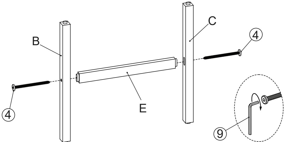
Attach the Leg Support Bar (E) to the Right Leg (C) and Left Leg (B) by using Screws (4) and Allen Wrench (9).
