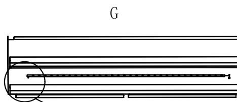
Note: Stick the LED strip on the bottom of the layer board, with the light facing downwards, to achieve a better lighting effect.
