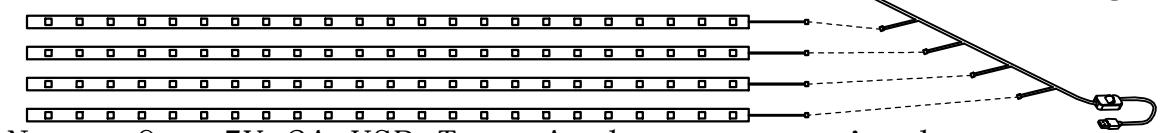
Note: One 5V 2A USB Type A charger required to power the LED light strip. (Not Included)
