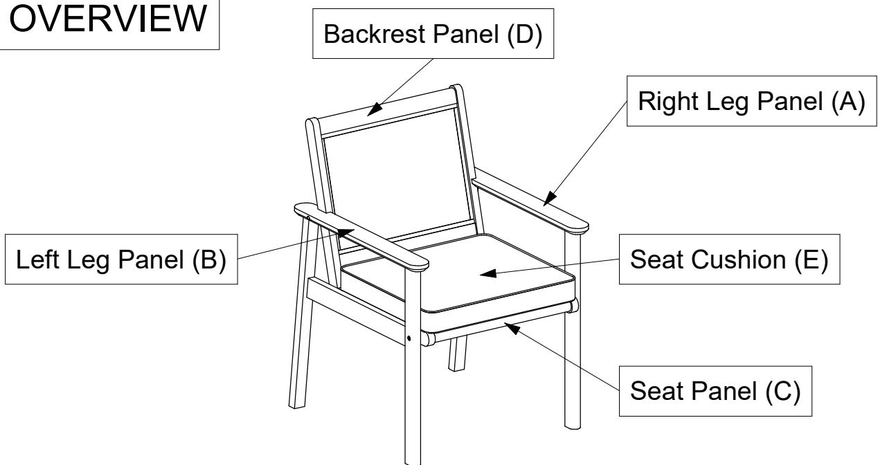
This Chair has multiple parts and may require up to some 30 minutes to assemble. To give you an overview of the Chair, the above picture is to help you put the various parts into perspective. Please read through the instructions here below to familiarise the parts and steps before assembly.
