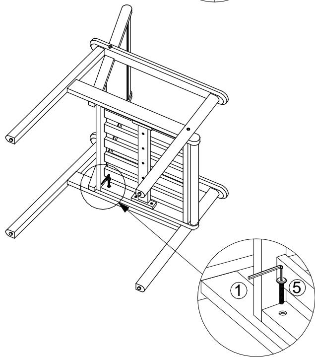
4.1. With assistance from your adult partners, attach Right Leg Panel (A) to Seat Panel (C) by using 1 Screw ( ) with Allen Wrench ( ) to secure. Attach Right Leg Panel (A) to Backrest Panel (D) by using 1 Bolt ( ) with Allen Wrench ( ) to secure as shown above picture.
