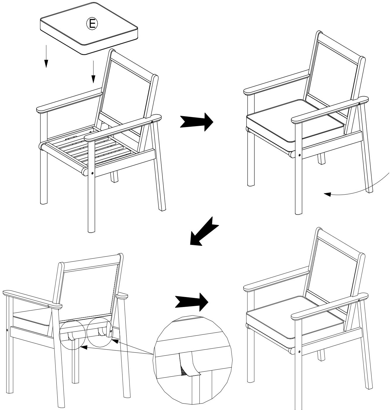
Place the Seat Cushion (E) on the seat of the Chair using the magic tape strap to secure as shown above.
